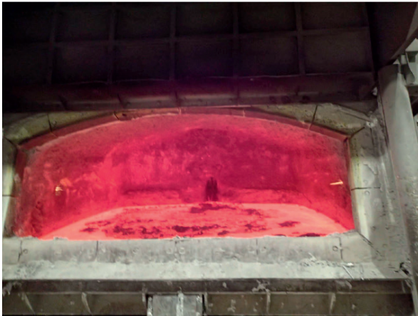
The figure shows an aluminium melting furnace with an aluminium melt covered with a (dark) dross layer. Ref: H. Fosshem, Alcoa Norway.
