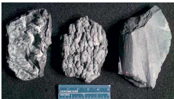
The figure illustrates scaling products from the electrolysis off-gas channel.
