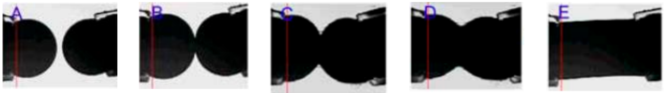
Figure: Route of coalescence of two oil droplets determined by a drop-bubble micropipette setup.
