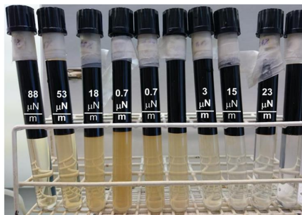
Figure: Phase behaviour of IFT of crude oil and solution of surfactant 0.068 and 0.410 mol/L NaCl (increasing form left to right). All IFT values are given in units of 10 -6 N/m.
