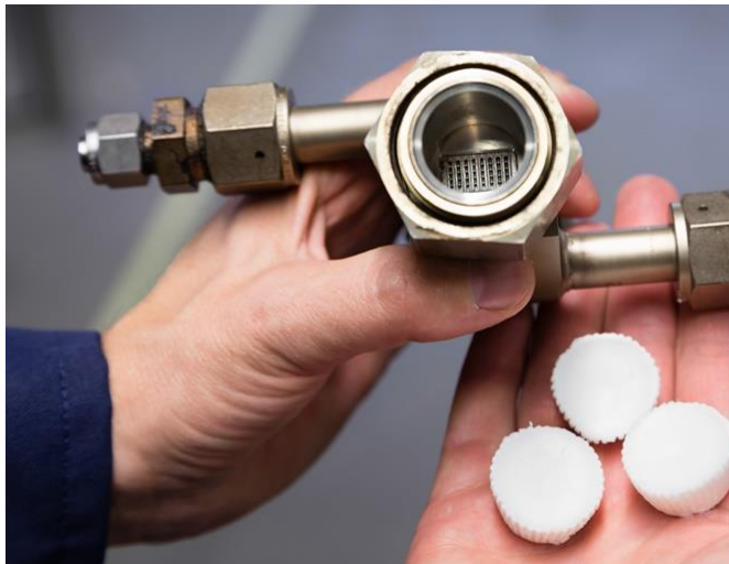
Examples of microstructured reactors (Photo: Thor Nielsen)
