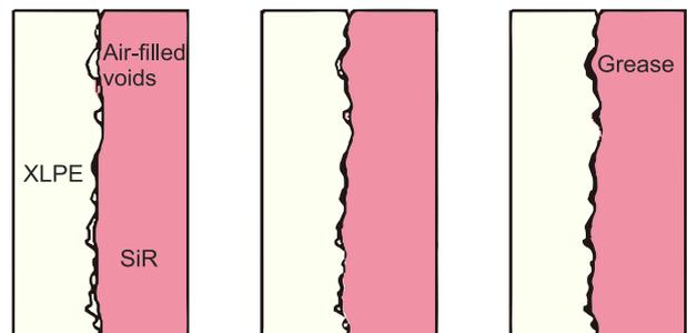
**Fig. 1** – The tribosystem: Interface between silicone rubber and XLPE [1]
