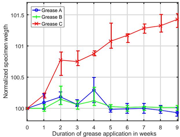
**Fig. 7** – Diffusion result of three different greases in SiR with interface pressure of about 5 bar
