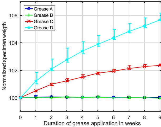
**Fig. 5** – Diffusion result of four different greases in SiR without pressure
