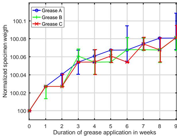
**Fig. 10** – Diffusion result of three different greases in EP without pressure
