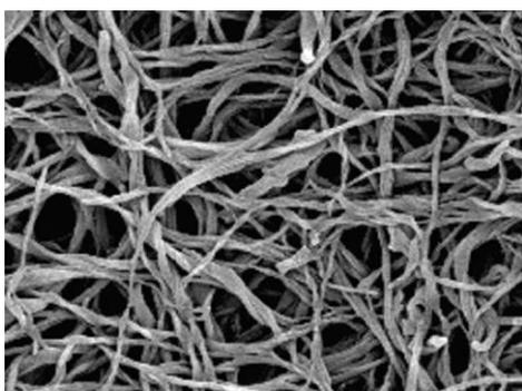
**Fig. 3** – Soap-like structure of the thickener [3]
