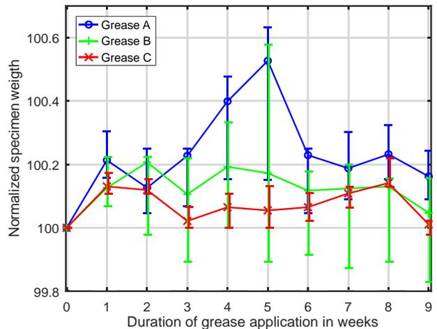
**Fig. 9** – Diffusion result of three different greases in XLPE without pressure
