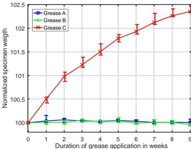
**Fig. 6** – Detailed diffusion result of three different greases in SiR without pressure
