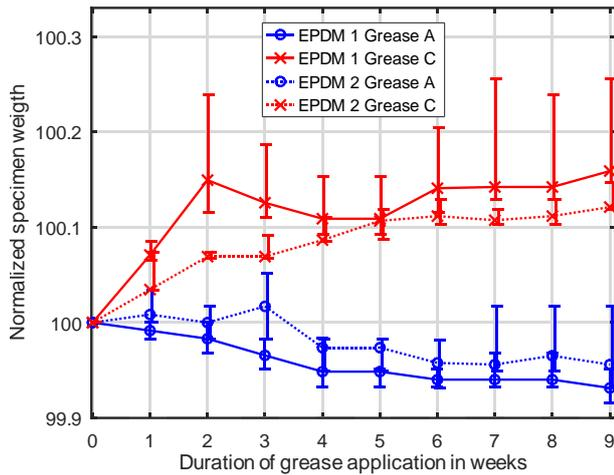
**Fig. 8** – Diffusion result of two different greases in two different EPDM rubbers without pressure
