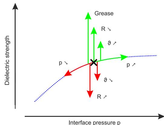
**Fig. 2** – Influence of the surface roughness of the XLPE (“R”), the interface pressure (“p”) and the temperature (“θ”) on the dielectric strength of the interface [1]
