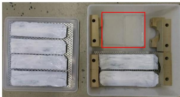
**Fig. 4** – Storage box for a set of six specimen with grease and the saturated salt solution to keep the air humidity constant (red marked in the top of the box)
