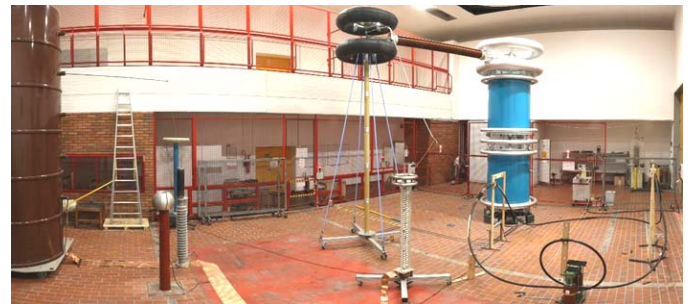
Figure 3. Arrangement for superimposed voltage test [8]
