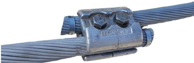
**Figure 2.** Clamp with bead-blasted conductors
