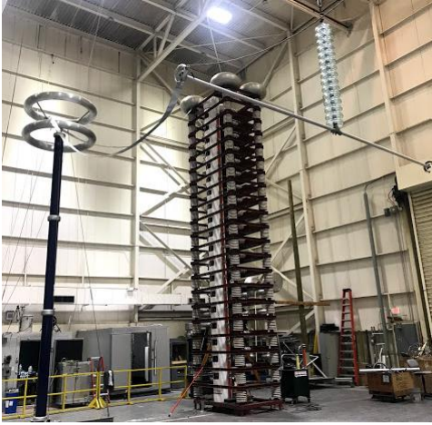
Figure 2. Test setup for up-and-down impulse measurements on glass insulator string.
