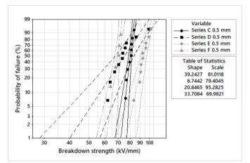
Figure 6. Breakdown strength on 0.5 mm test objects using semispherical electrodes an in oil 2 with (Series D, E, and F) and without (Series C) silicone embedded electrodes.
