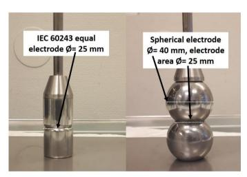
Figure 1. Electrode system according to IEC 60243 to left and partially-spherical electrodes to right.
