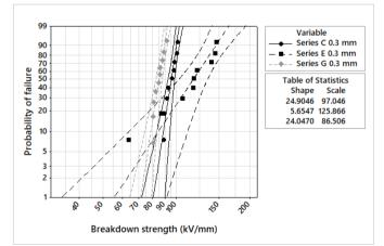
**Figure 7.** Breakdown strength on 0.3 mm test objects using semispherical electrodes in oil 1 and 2 with and without silicone 2, where the combination of oil 2 and silicone 2 (Series E) has combined effect on the breakdown strength compared oil 1 and silicone 2 (Series G).
