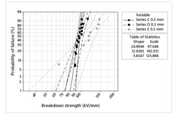
Figure 5. Breakdown strength on 0.3 mm test objects using semispherical electrodes an in oil 2 with (Series D and E) and without (Series C) silicone embedded electrodes.
