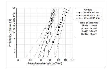
**Figure 8.** Breakdown strength on 0.5 mm test objects using semi spherical electrodes an in oil 1 and oil 2 with and without silicone 2, where the combination of oil 2 and silicone 2 (Series E) has a combined effect on the breakdown strength compared oil 1 and silicone 2 (Series G).
