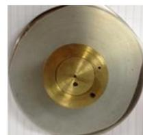
**Figure 2.** A typical sample on the high voltage electrode and current measurement- and guard electrode mounted on the sample. The area of the measurement electrode is  $7.1 \text{ cm}^2$ .
