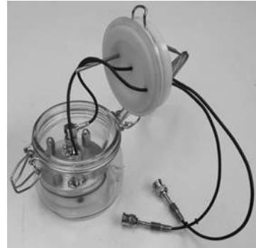
Fig. 2 – Electrode system in a hermetic container
