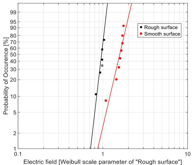
Figure 8 Weibull plot of breakdown measurement results normalized by Weibull scale parameter ( $\alpha$ ) of curve "Rough surface".
