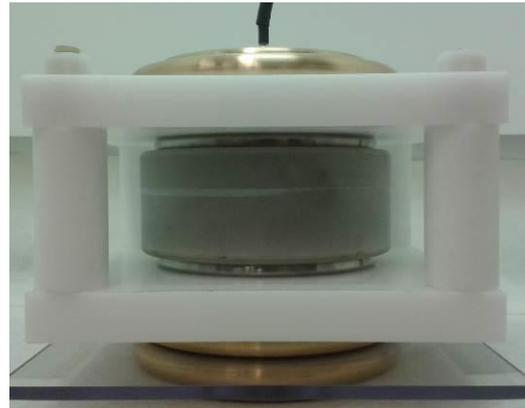
Figure 3 Photo of mounted inner part of test cell prior to gel filling.
