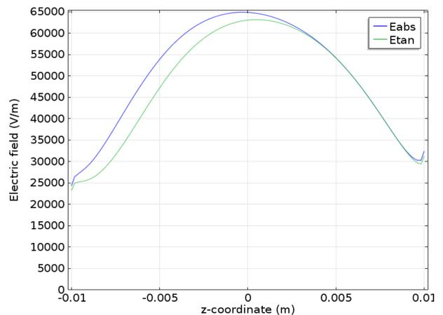
Figure 6 Simulated electric field in rubber-epoxy interface at applied voltage 1 kV peak. Absolute field (Eabs) and tangential field (Etan).
