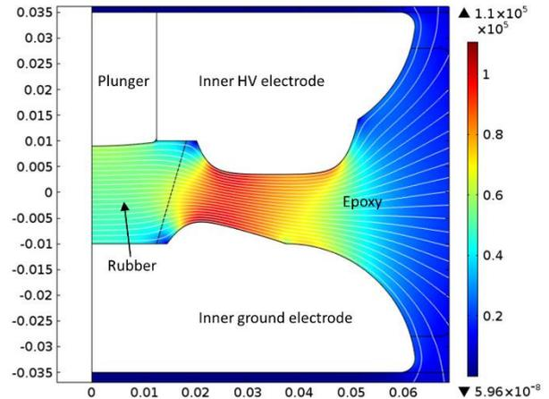
Figure 5 Simulated electric field distribution (color) and equipotential lines in inner part of test cell. Applied voltage 1 kV peak. Plunger extending 1 mm into rubber plug.
