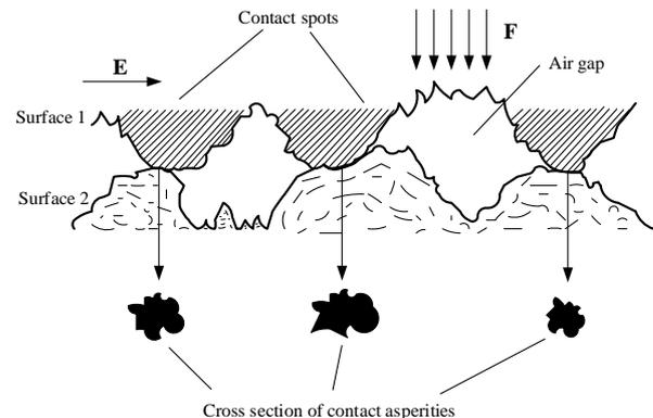
Fig. 2 – Schematic illustration of a solid-solid interface consisting of contact spots and asperities.
