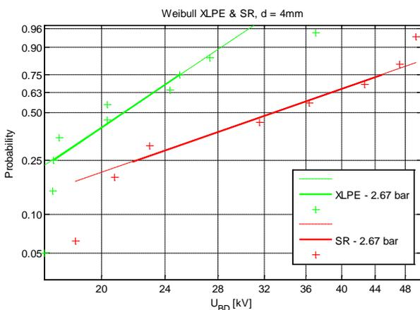
**Fig. 9** – The Weibull plot of measured AC breakdown voltage of XLPE-XLPE interface vs. SR-SR interface at 2.67 bar.
