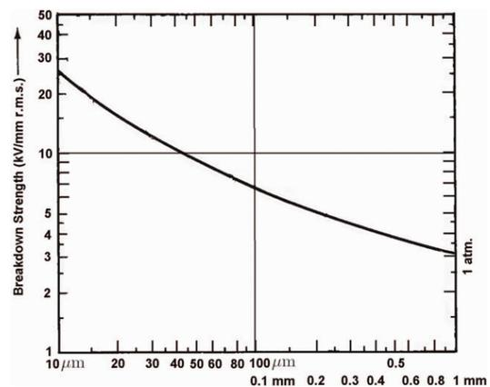
Fig. 3 – Breakdown strength of spherical air gaps as a function of the electrode gap.
