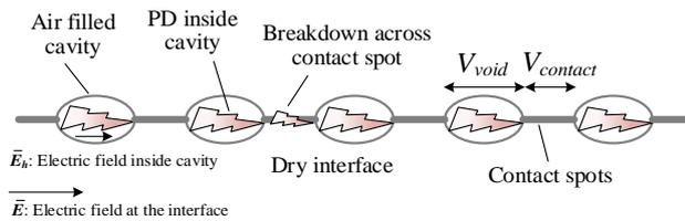
**Fig. 4** - The electrical model of voltage drop at the interface.
