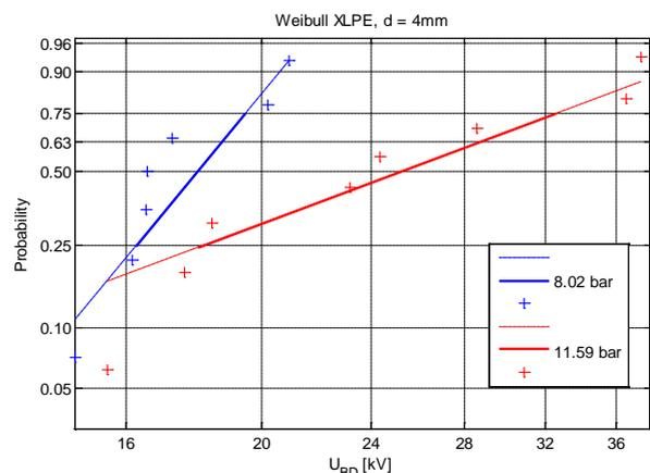
**Fig. 7** – The Weibull plot of measured AC breakdown voltage of XLPE-XLPE interface.
