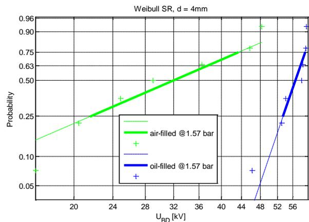
**Fig. 10** – The Weibull plot of measured AC breakdown voltage of SR/SR interface at 1.57 bar (air-filled vs. oil-filled voids).
