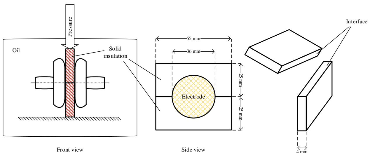
**Fig. 5** – Sketch of the experimental setup with the samples mounted between the Rogowski electrodes.
