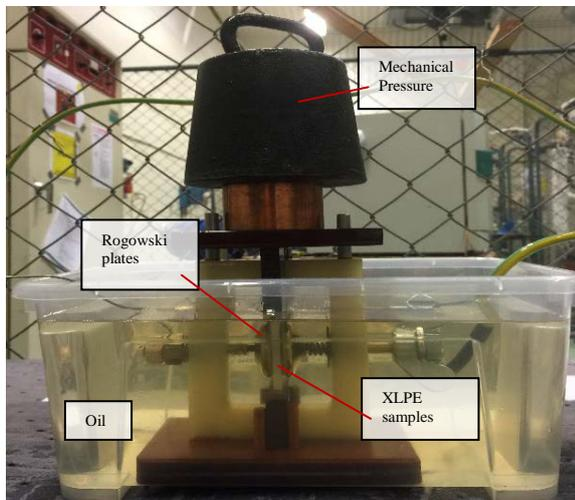
**Fig. 6** – Experimental setup of Rogowski electrodes with samples attached and mechanical pressure applied.
