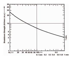
**Fig. 3** – Breakdown strength of spherical air gaps as a function of the electrode gap.
