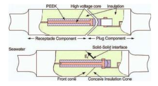
Fig. 1 – Illustration of wet-mateable connector design [1].
