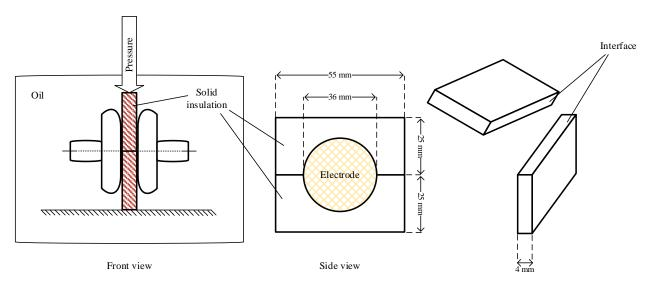
Fig. 5 – Sketch of the experimental setup with the samples mounted between the Rogowski electrodes.
