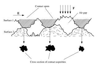
**Fig. 2** – Schematic illustration of a solid-solid interface consisting of contact spots and asperities.
