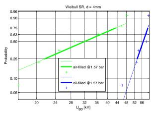
**Fig. 10** – The Weibull plot of measured AC breakdown voltage of SR/SR interface at 1.57 bar (air-filled vs. oil-filled voids).
