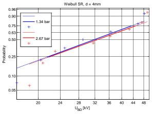
Fig. 8 – The Weibull plot of measured AC breakdown voltage of SR-SR interface.
