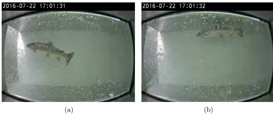
Figure 5: Example of how air bubbles influence the frames. The two frames are from the same video of the same trout. When the fish is at the top of the frame occluding air bubbles can influence the classification. Less occlusion is present when the fish is closer to the center.
