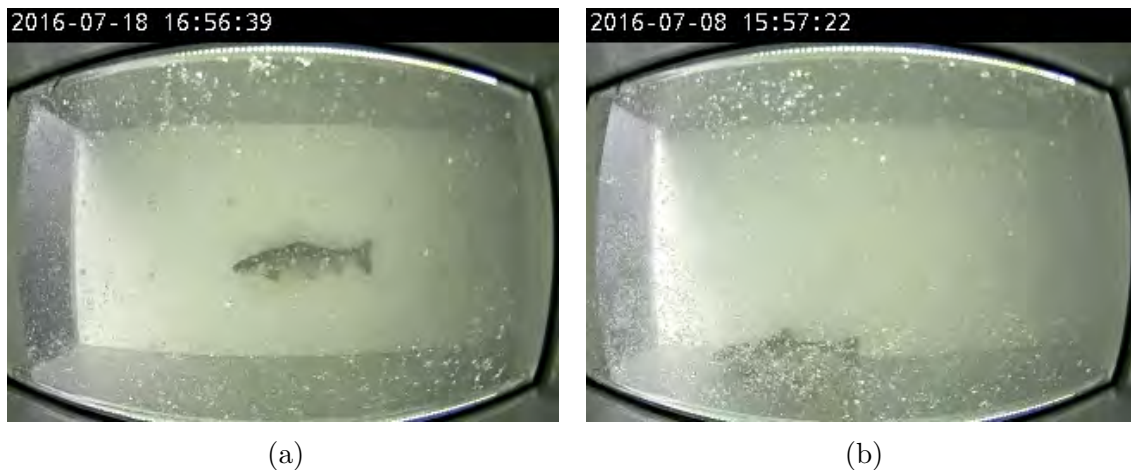
Figure 2: Example images. A smaller trout on the left without occluding air bubbles, and on the right a smaller trout with many occluding air bubbles. It is clear that air bubbles can influence the classification.
