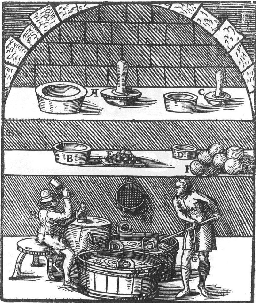
Figure 5.3. The different stages in cupel production. A and C are moulds and stamps for cupels, B and D are cupels made from A and C, E is a stack of cupels, F are balls of washed ashes, G shows a man washing ashes and H shows a man pounding cupels. A sieve is hanging on the wall. Reproduced from Lazarus Ercker's treatise ((1574)1951:32).
