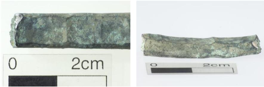
*Figure 5.5. Pictures of the thick rod N125026. It is the lightest rod and broken in both ends. Note the wavy appearance of the surface, whilst the opposite surface is smooth. This indicates hammering with a larger hammer over a cylindrical anvil. Photograph by Bruce Sampsson, NTNU Vitenskapsmuseet*
