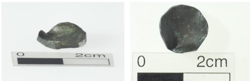
*Figure 5.11. Blank N119889b (period 6 / phase 3) from two perspectives. Note the bowl shaped appearance, some straight sides and the hammered corners. This is due to cutting of corners before hammering a pile of blanks. Microstructures see figure 5.12. Photograph by Bruce Sampson, NTNU Vitenskapsmuseet.*
