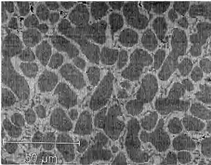
*c) Cast in a sand mould*
