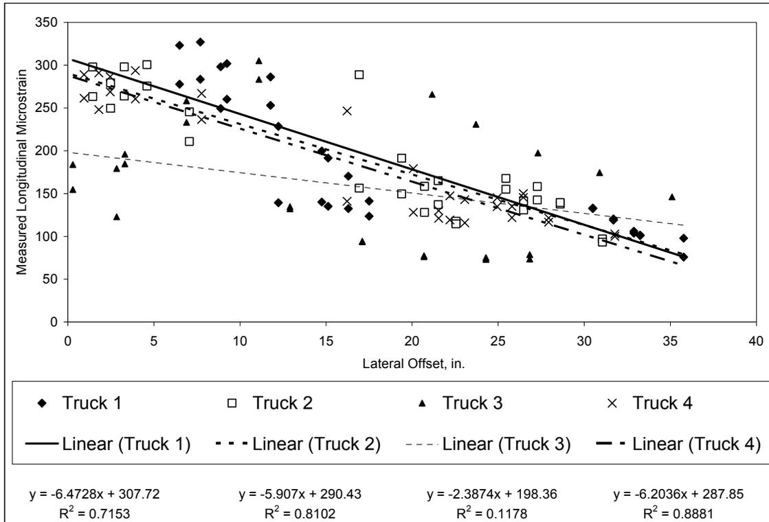
Figure 10: Effect of lateral offset on strain response.
