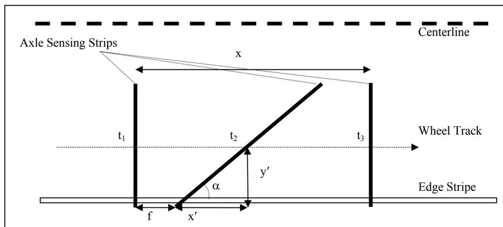
Figure 2: Arrangement of axle sensing strips.
