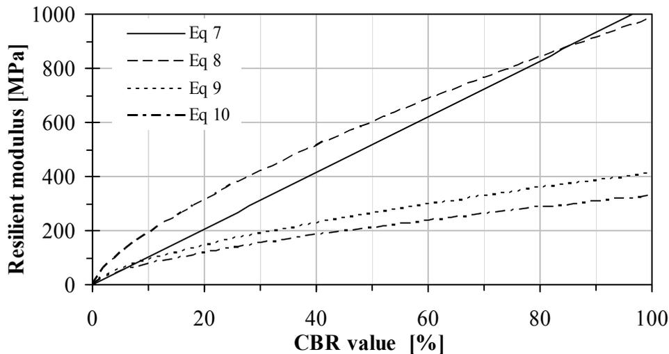
Figure 2: Predicted stiffness values as a function of CBR values according to the equations in Table 1.
