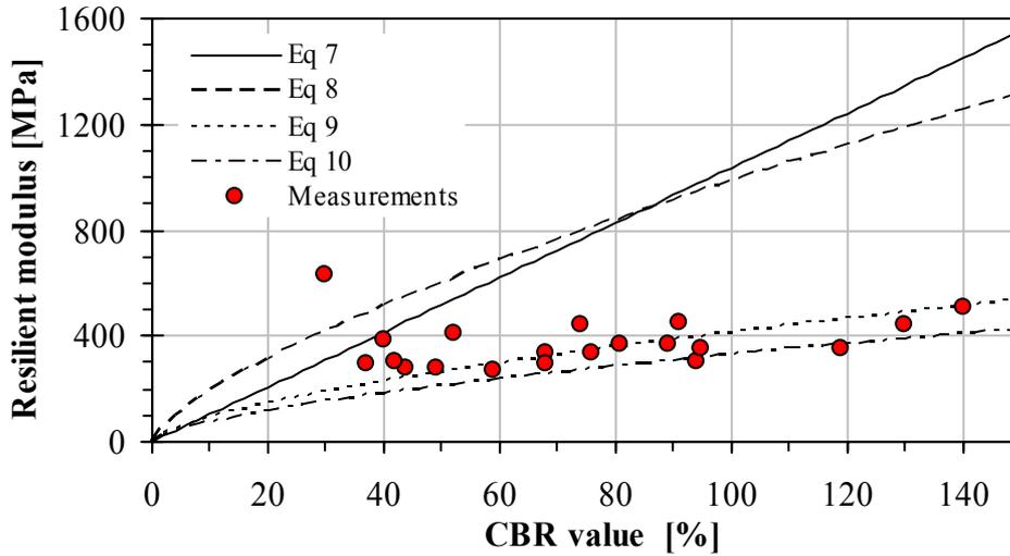
Figure 7: Predicted resilient modulus based on the CBR value from the four equations in Table 1 as well as the measured stiffness from the RLT test measurements at the mean stress level  $p = 250$  kPa.
