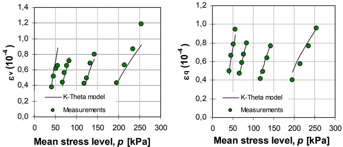
Figure 4: Typical results from RLT testing: comparison of measured and calculated strains. a) volumetric strain and b) deviatoric strain versus the mean applied stress level.
