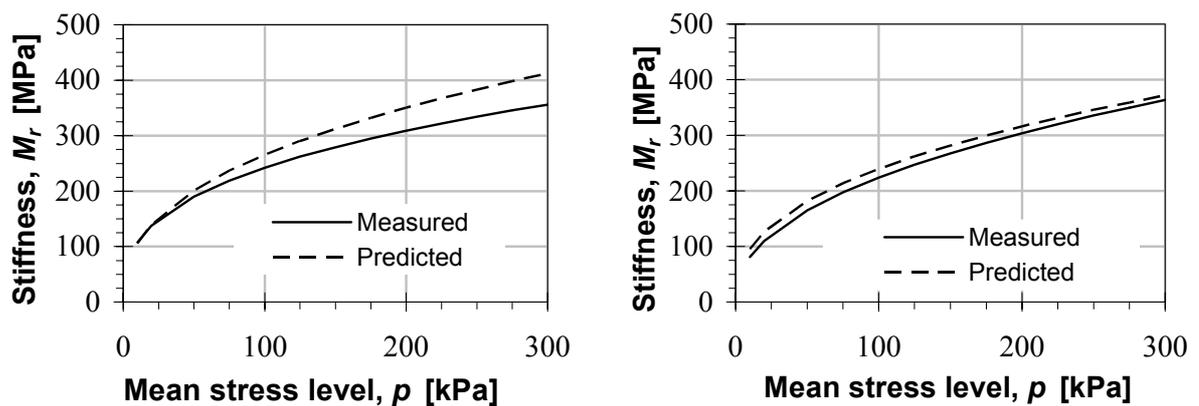
Figure 8: Resilient modulus versus mean stress level for two materials based on actual  $k_1$  and  $k_2$  values and  $\hat{k}_1$  and  $k_2 = 0.4$  respectively. a) the Raudamelur material with  $\Delta = -14.7\%$  and b) the Jökulsa a Dal material with  $\Delta = -3.0\%$ .
