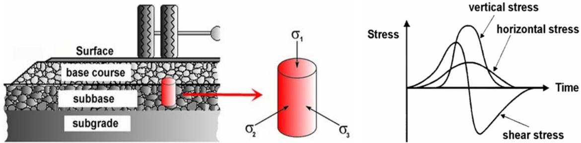
Figure 1: Stresses in a UGM layer. a) Typical pavement structure and stresses, b) induced stresses in a pavement element due to moving wheel load.
