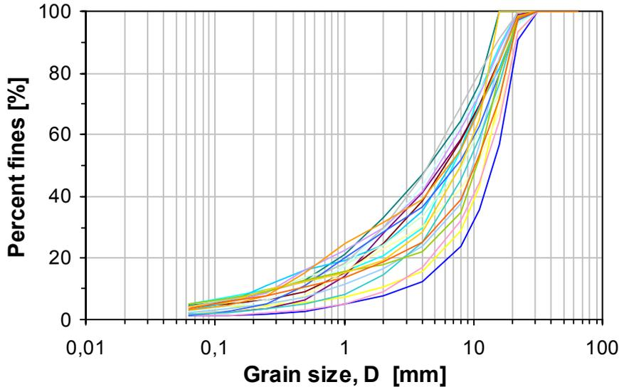
Figure 5: Overview of the grain size distribution of the twenty materials used in this study.
