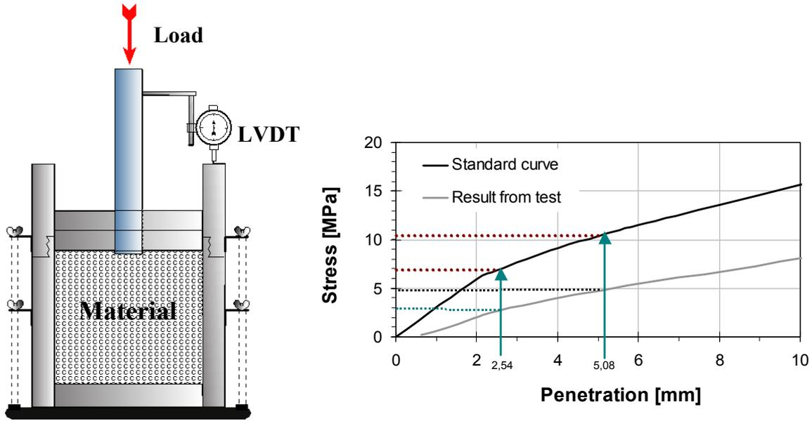
Figure 3: CBR test set-up and a schematic view of the evaluation of the CBR value.
