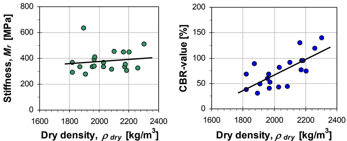
Figure 6: Measured maximum stiffness at mean stress level  $p = 250$  kPa and CBR value as a function of dry density for all the twenty materials.
