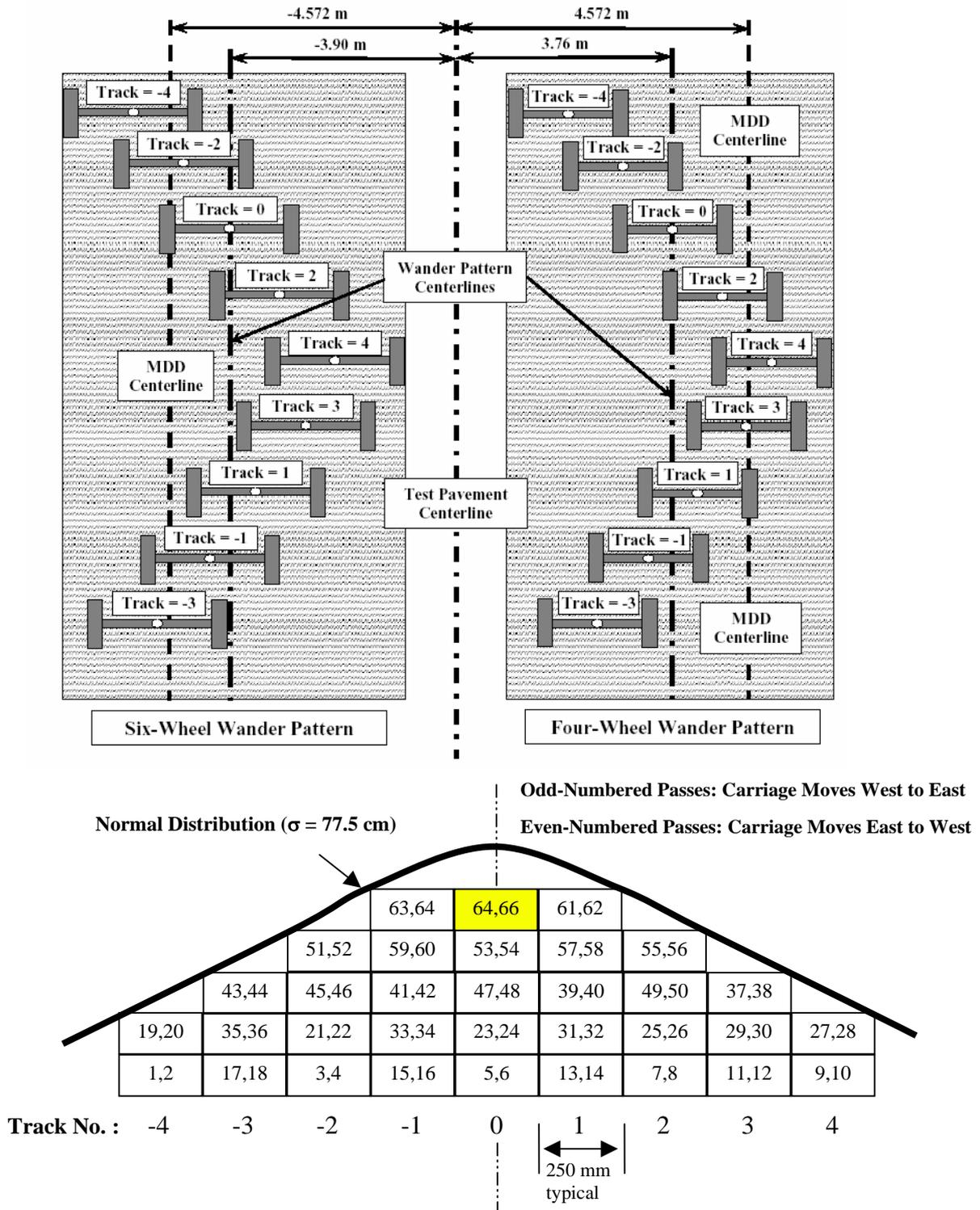
Figure 1: Applied traffic wander patterns and wander distributions in the NAPTF tests
