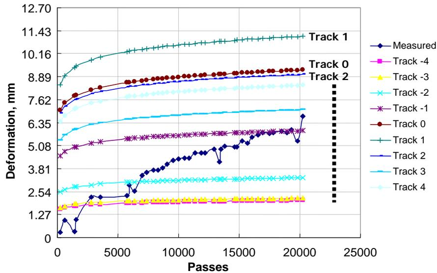
Figure 3: Individual wander position (or track) permanent deformations predicted at the MDD centerline location in the LFC P154 subbase layer
