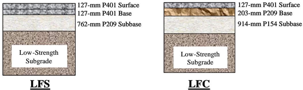
Figure 2: The NAPTF pavement cross-sections of LFS and LFC test sections
