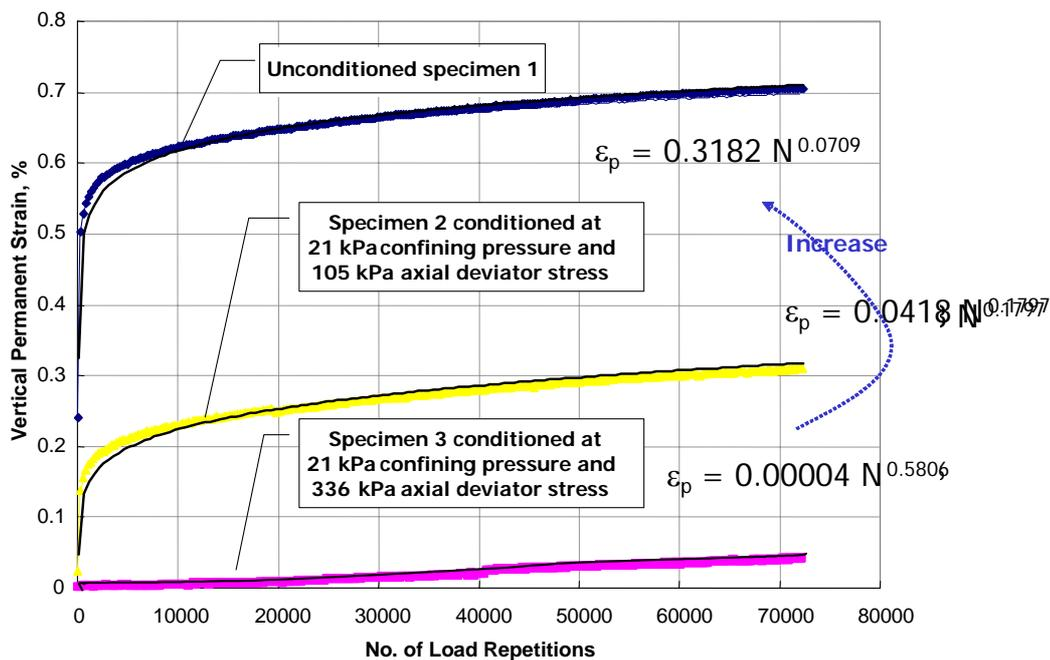
Figure 7: Illustration of stress history effect on the specimen permanent strain accumulation
