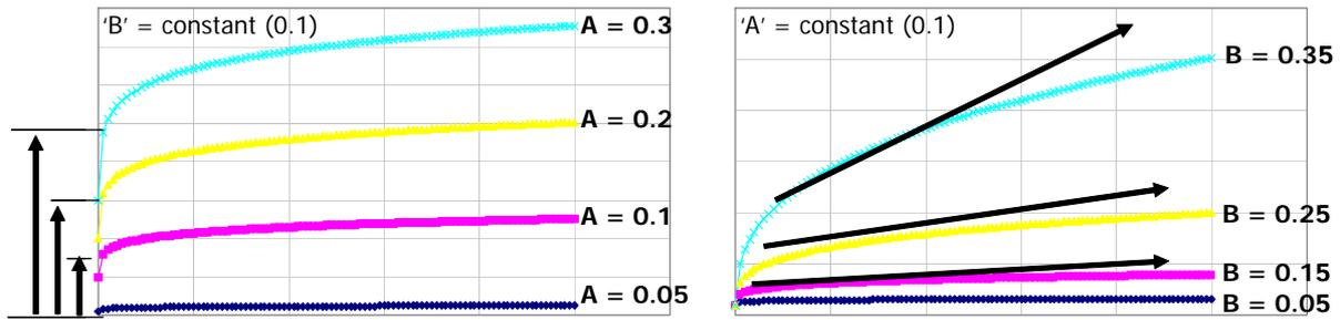
Figure 5: Effects of 'A' and 'B' parameters on the  $\epsilon_p = A*N^B$  power function type model
