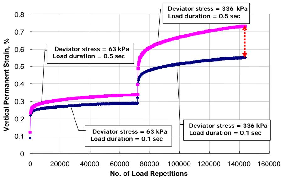
Figure 6: Illustration of load duration effect on the specimen permanent strain accumulation
