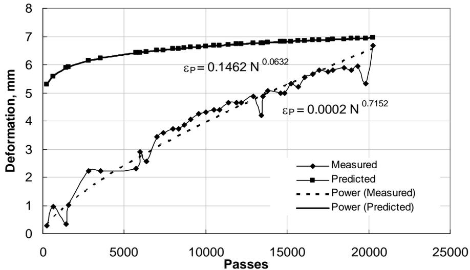
Figure 4: Measured and predicted permanent deformations in the LFC P154 subbase layer
