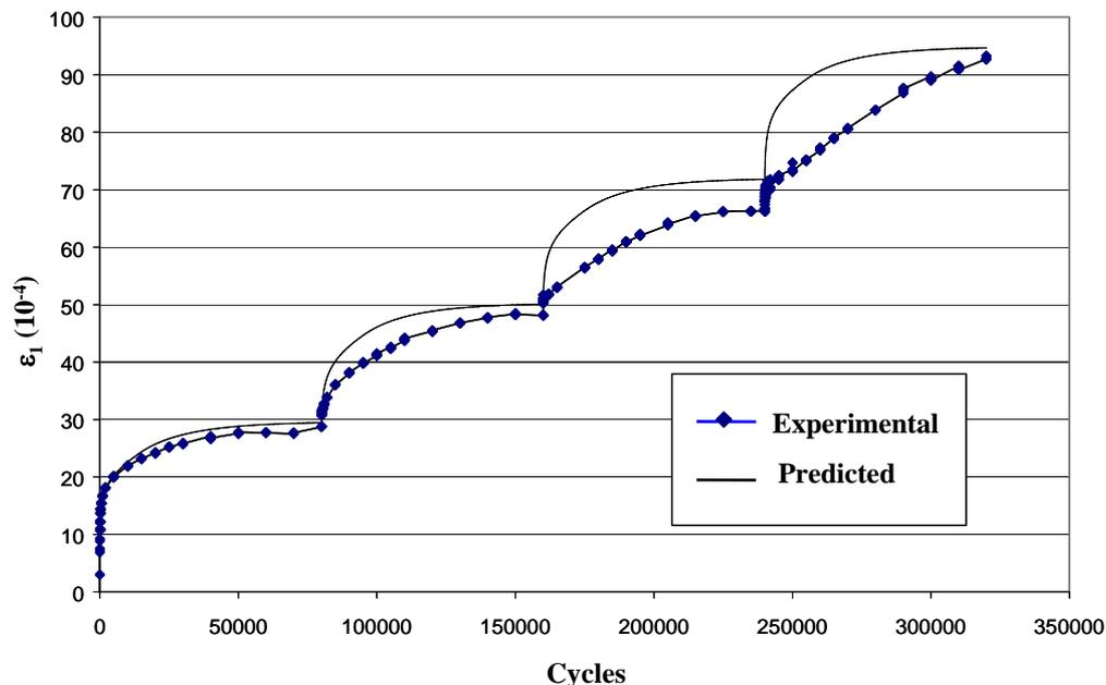
Figure 8: Predicted and measured unbound aggregate permanent strains (El abd et al., 2004)
