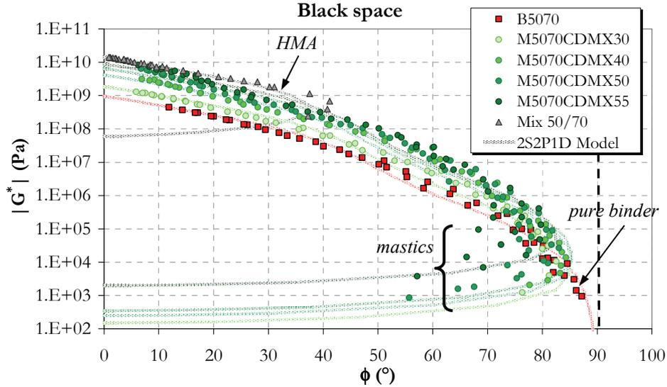
Figure 9. Complex modulus in Black space of bitumen 50/70, 4 mastic formulations based on CDMX filler (30%, 40%, 50% and 55%), and Hot Mix Asphalt (HMA).
