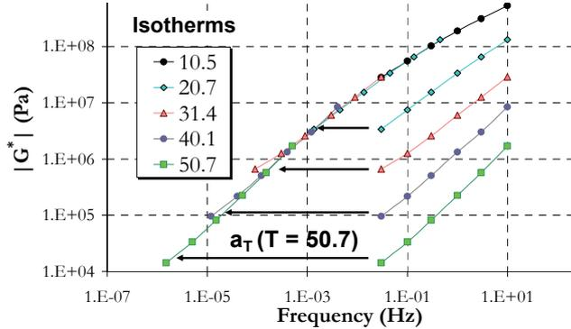
Figure 5. Construction of a master curve with  $a_T$  factor (temperature in °C).
