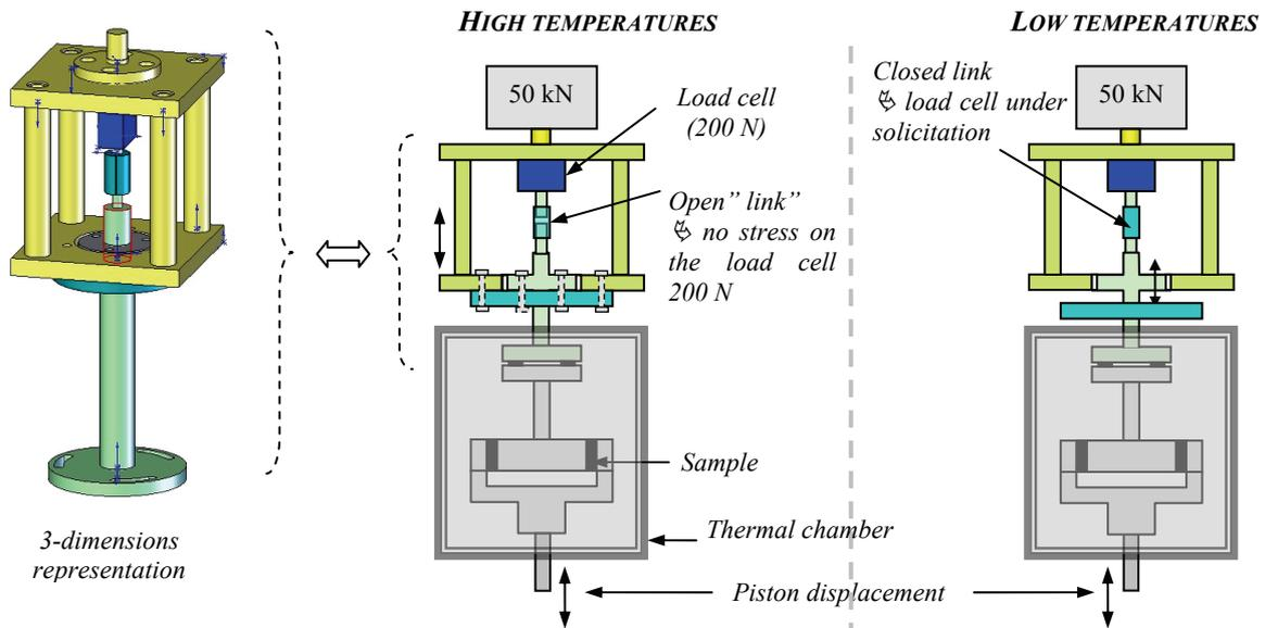
Figure 2. Schematic view of the by-pass system to make transition between low temperature measurements and high temperature measurements
