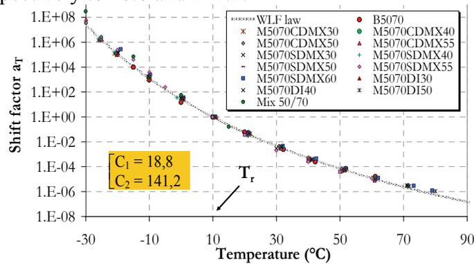
Figure 6. Shift factor  $a_T$  of all the tested materials formulated from the binder, at  $T_r = 10^\circ\text{C}$ .
