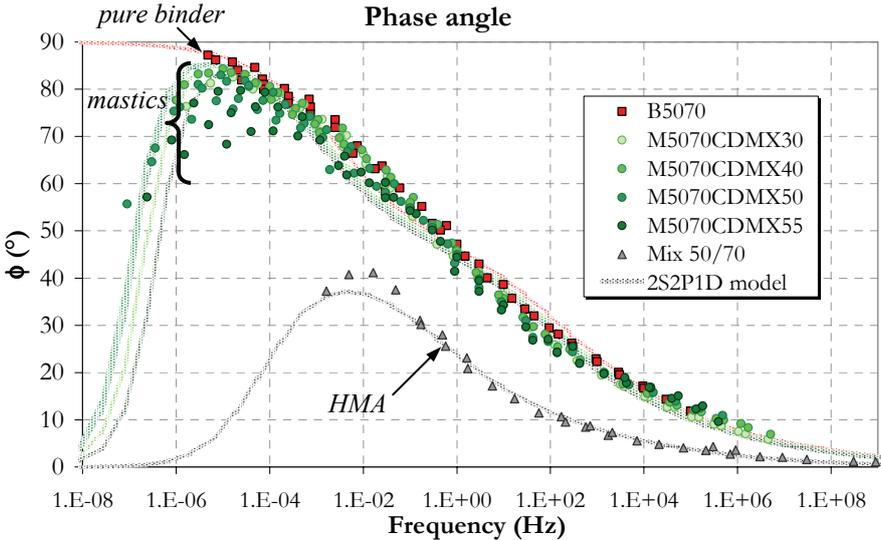
Figure 8. Phase angle master curves of bitumen 50/70, 4 mastic formulations based on CDMX filler (30%, 40%, 50% and 55%), and Hot Mix Asphalt (HMA). 2S2P1D Model.
