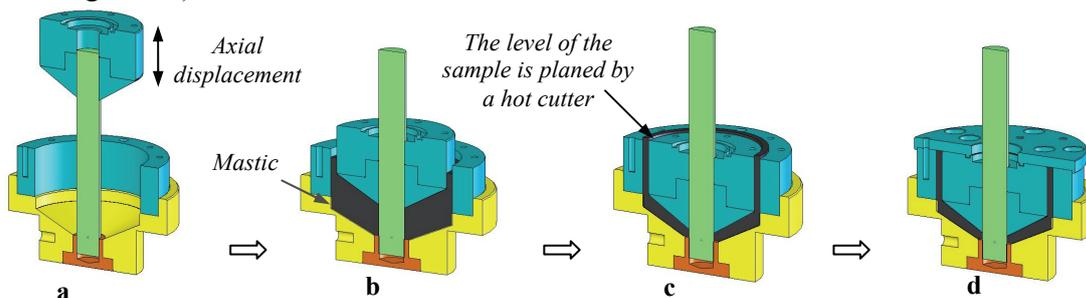
Figure 3. Schematic of moulding of high filler content mastics
