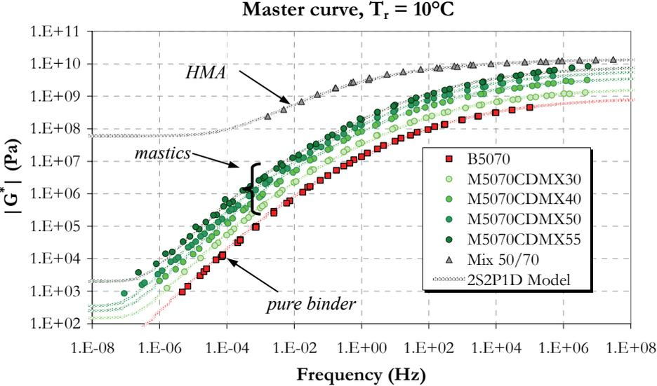
Figure 7. Modulus master curves ( $T_r = 10^\circ\text{C}$ ) of bitumen 50/70, 4 mastic formulations based on CDMX filler (30%, 40%, 50% and 55%), and Hot Mix Asphalt (HMA). Straight lines are simulation with the 2S2P1D model (cf. section 4.3)
