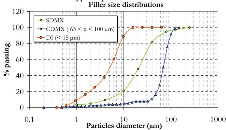
Figure 4. Particle size distribution of the different filler types
