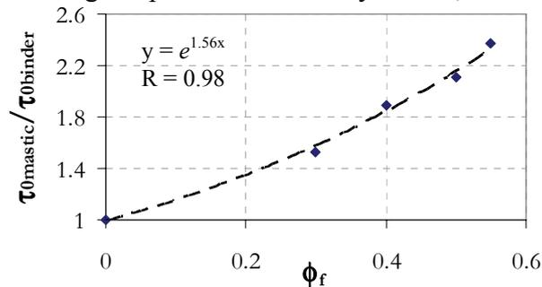
Figure 11. Evolution of the characteristic time of mastics as a function of the filler content
