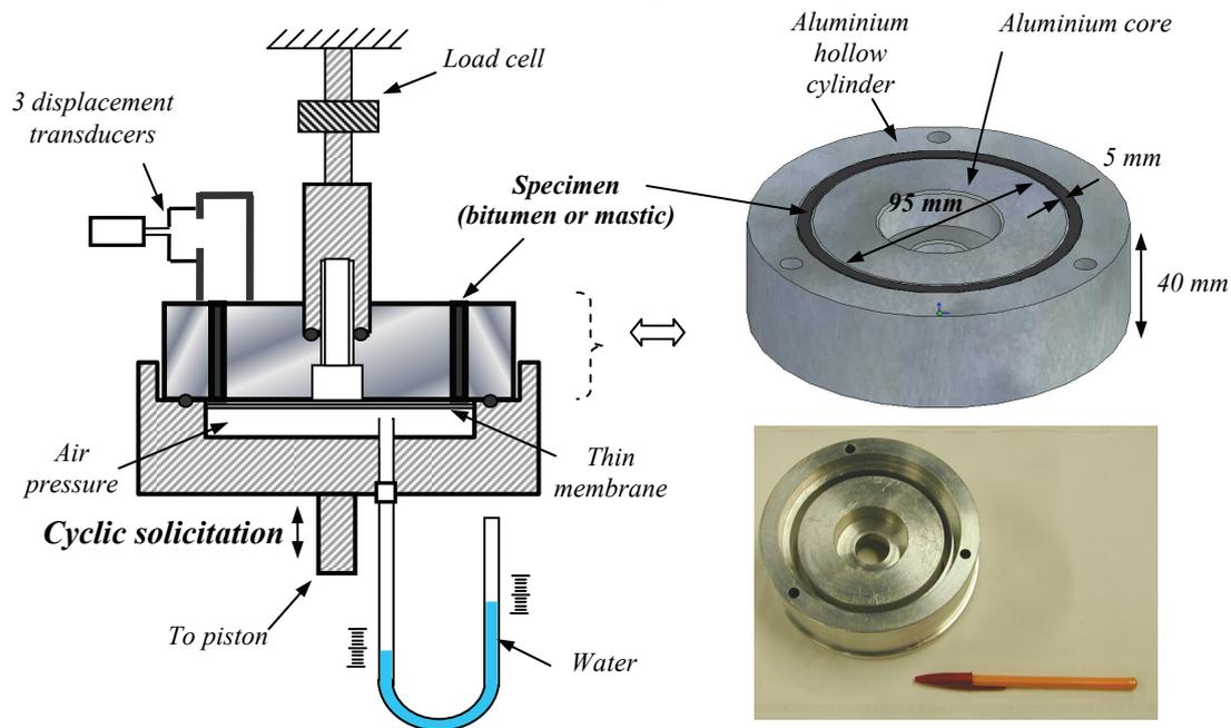
Figure 1. Schematic of the new annular shearing rheometer for bitumen and mastic
