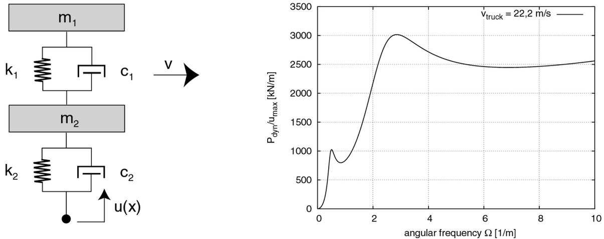
Figure8: Two mass dashpot-spring-system (left) and corresponding amplification function for a driving velocity of  $v = 80$  km/h (right)
