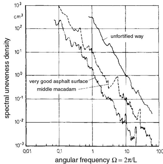
Figure2: Measured spectral unevenness density  $\Phi_h$  for different road types in dependency of the angular frequency  $\Omega$  (Mitschke, 1984)
