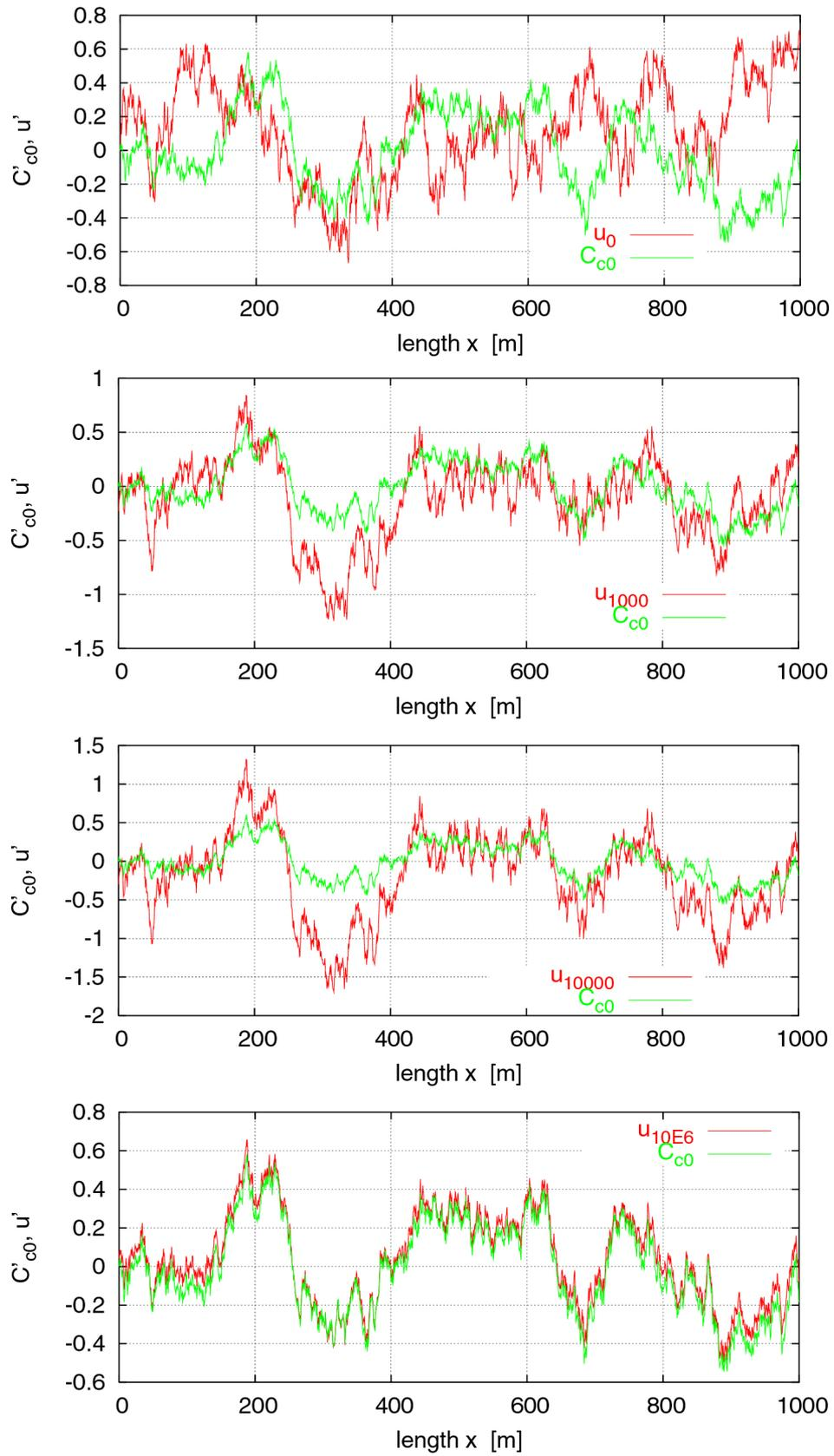
Figure9: Scaled variation of initial subsoil stiffness and scaled variation of unevenness for different load cycles
