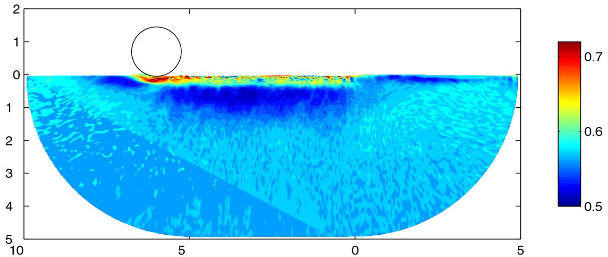
Figure6: Calculated void ratio after one pass with a vibratory roller, Kelm (2004)
