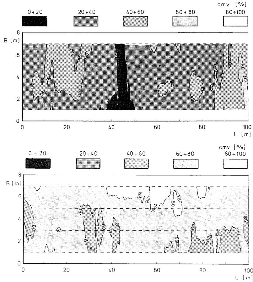
Figure3: Measured data cmv at the formation (top) and at the frost protection layer (bottom)
