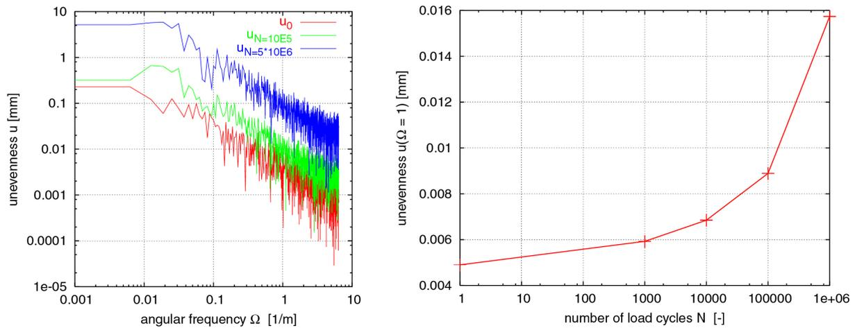
Figure10: Unevenness  $u$  as a function of angular frequency  $\Omega$  for different load cycles (left) and unevenness  $u$  for the angular frequency  $\Omega = 1$  as a function of load cycles (right)
