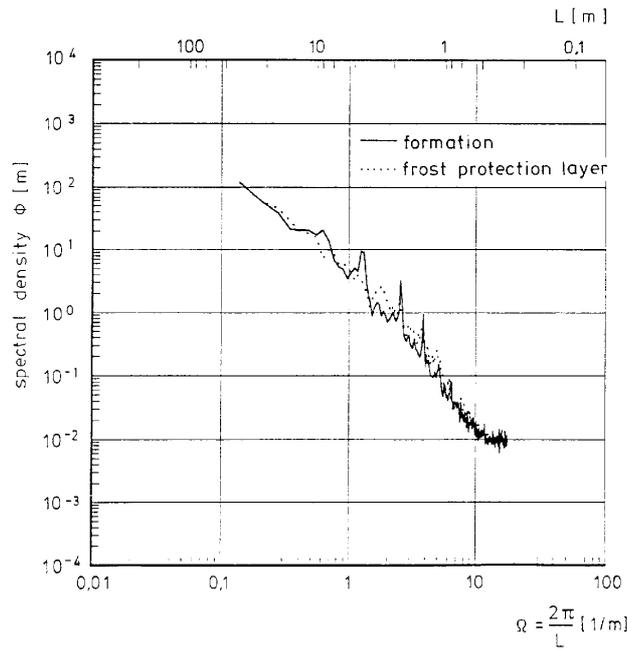
Figure4: Power spectral density  $\Phi$  as a function of wave length  $L$  and angular frequency  $\Omega$  at the formation and at the frost protection layer
