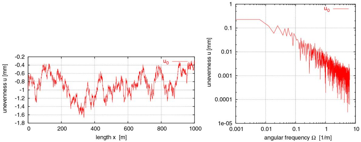
Figure5: Unevenness  $u$  of a young road (left) and unevenness  $u$  as a function of angular frequency  $\Omega$  (right)
