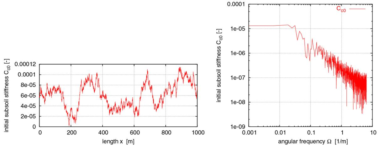
Figure7: Initial stiffness of subsoil  $C_{c0}$  (left) and initial stiffness of subsoil  $C_{c0}$  as a function of angular frequency  $\Omega$  (right)
