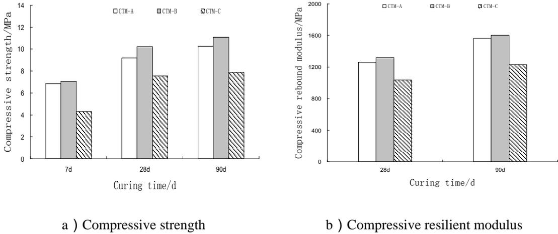
Figure2: Strength and modulus of cement stabilized aggregate with different structure types.
