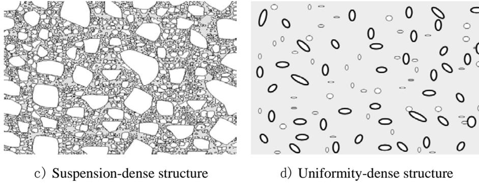
Figure1: Base material structure types.
