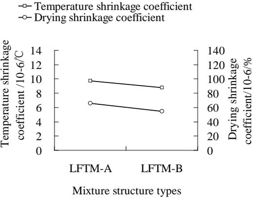
Figure6: Shrinkage coefficient results of lime fly-ash stabilized aggregate.
