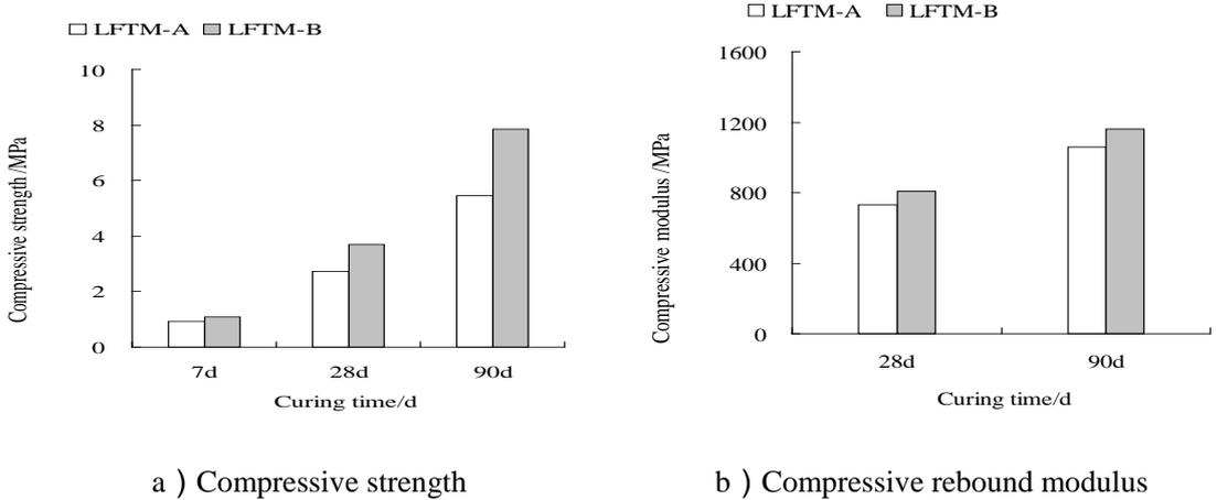
Figure5: Compressive strength and modulus of lime and fly-ash stabilized aggregate.
