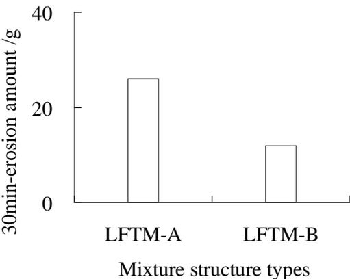
Figure7: Anti-erosion test results of lime fly-ash stabilized aggregate.
