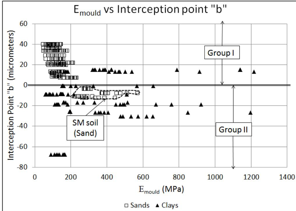
Figure 3: Interception point (b) vs. Back-calculated modulus in the mold ( $E_{mold}$ )
