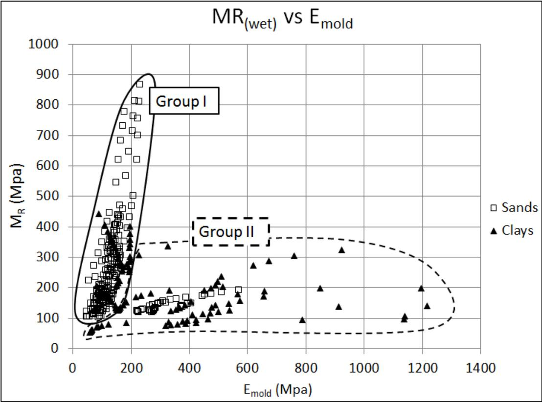
Figure 2: Resilient modulus ( $M_{R(wet)}$ ) vs. back-calculated modulus in the mold ( $E_{mold}$ )
