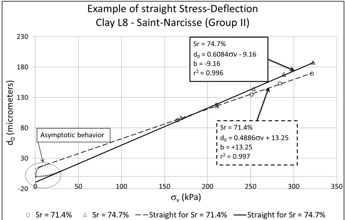
Figure 4: Example of straight stress-deflection line for a Group II soil (Clay L8 – Saint-Narcisse)
