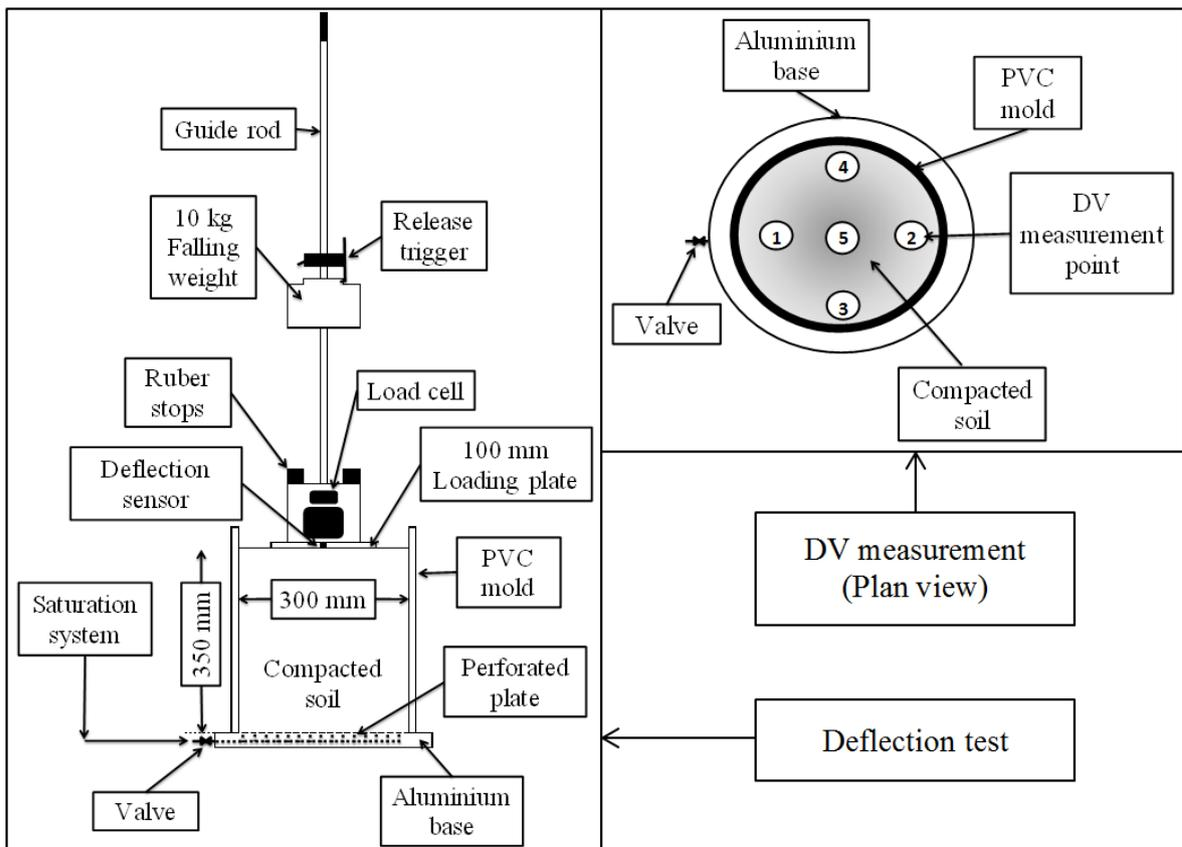
Figure 1: Deflection test with LWD and Dielectric Value measurements
