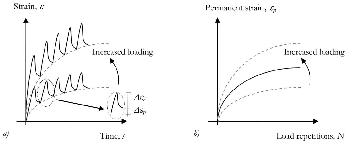
Figure 1: Effects of number of load applications and increased loading on development of the permanent strain (Erlingsson, 2010).
