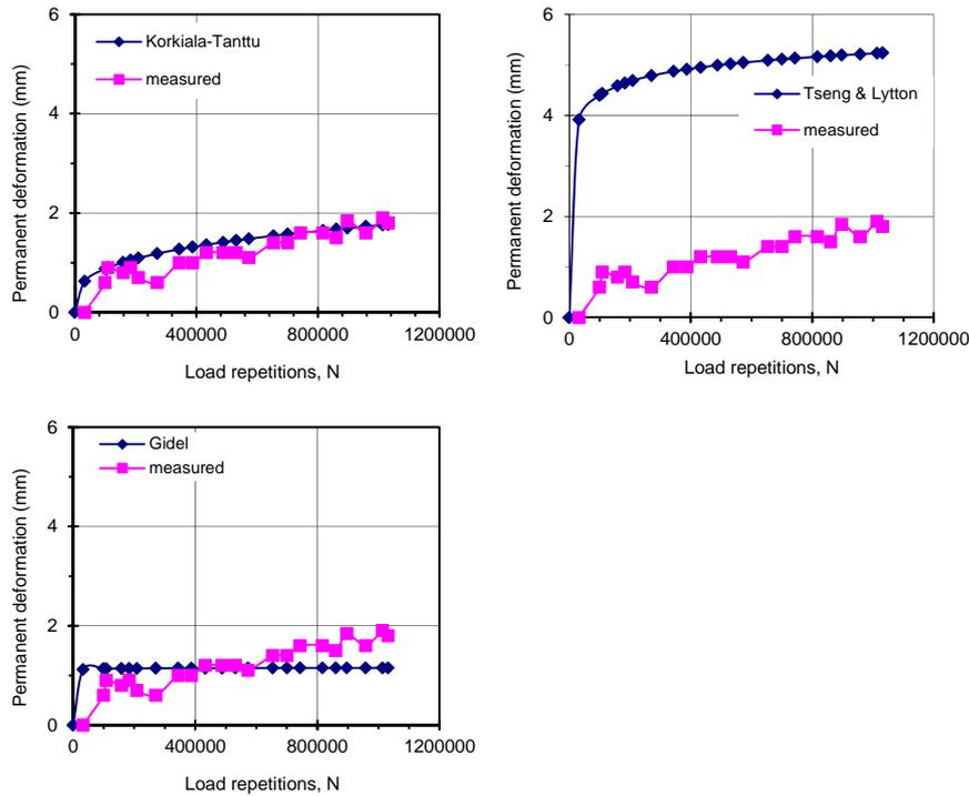
Figure 11: The results of comparisons between measured and calculated values of the permanent deformation in base course for three different models
