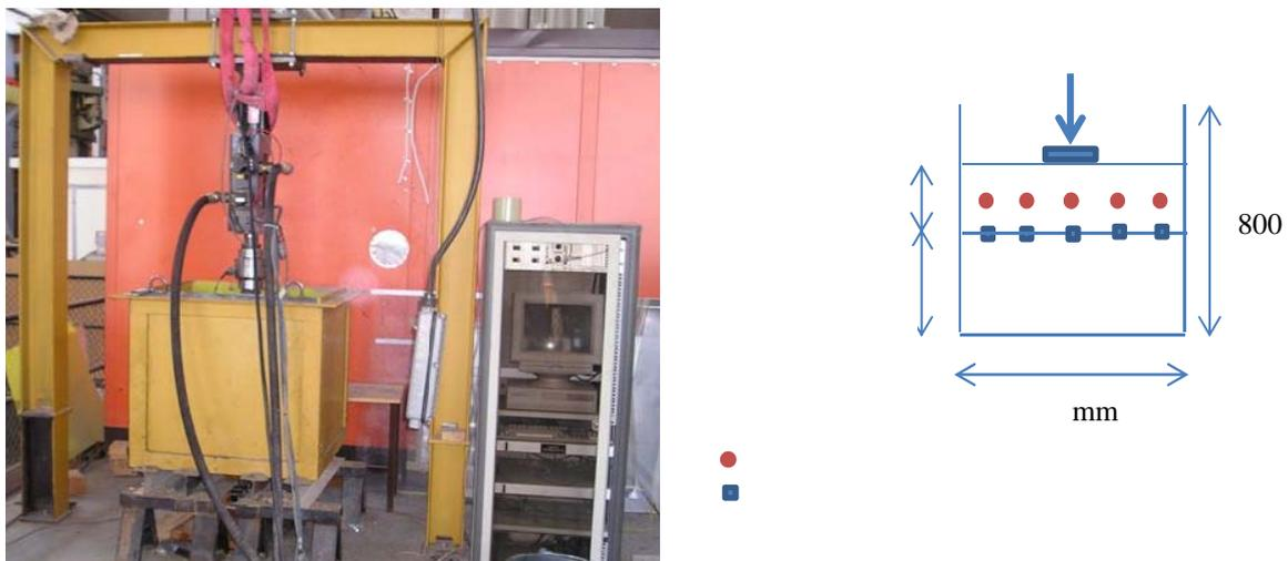
Figure 4: a) The testing box along with the loading and control unit. b) Five deformation gauges within the base course material and five at the top of the subbase.
