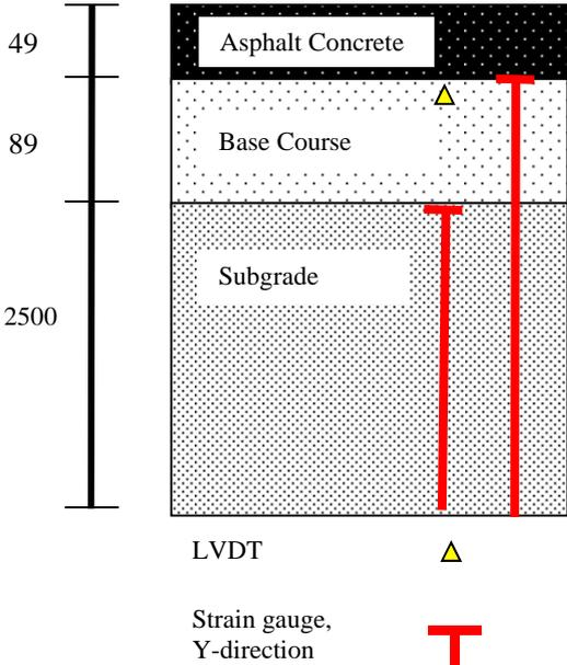
Figure 10: The test structure used in HVS-SE01 with instruments placed at different levels
