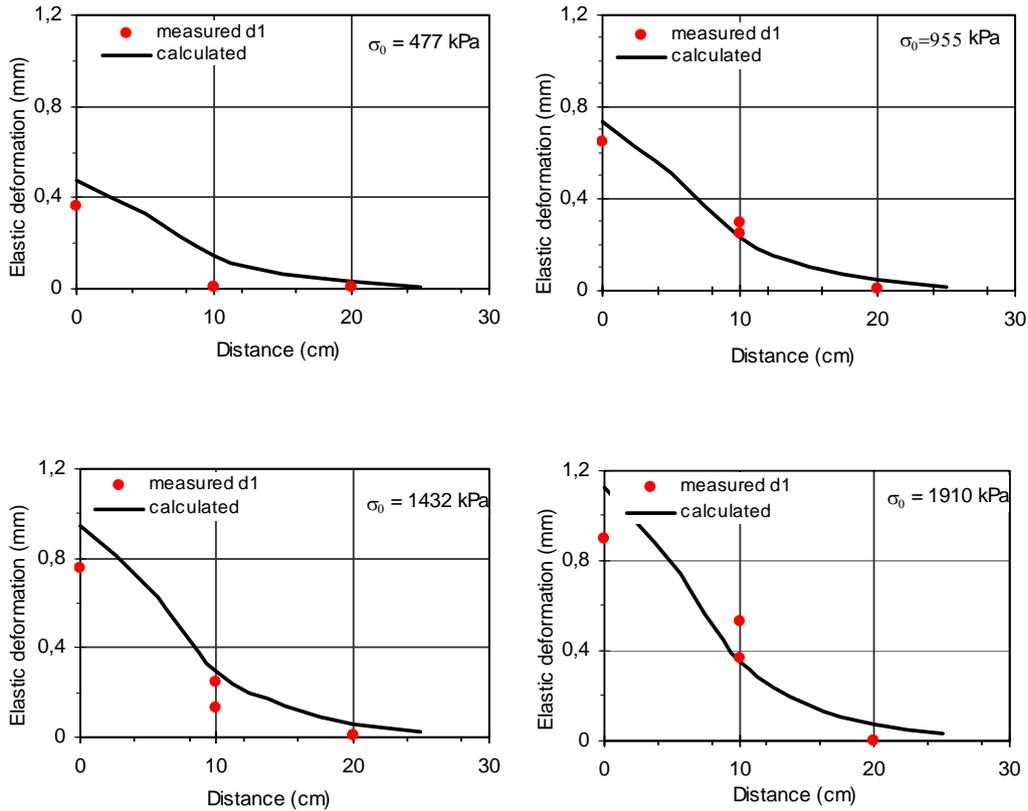
Figure 8: Comparison between numerical model (Non-linear) and the measurements from the testing box for material  $d_1$  in the middle of base course with four different vertical stresses and loading plate of 100 mm.
