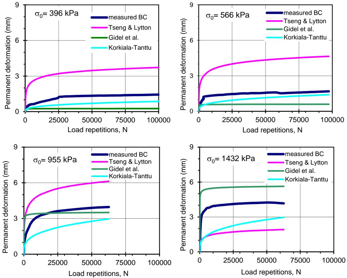
Figure 9: Measured and calculated accumulated permanent deformation as a function of the number of load repetitions of different surface loading in the middle of the base course.
