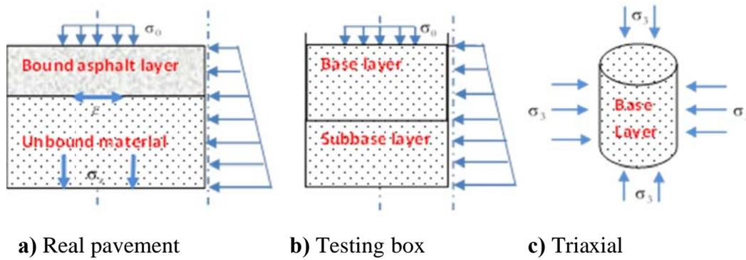
Figure 2: Variation of confining pressure in a) real pavement and laboratory simulation with b) testing box and c) triaxial testing specimen (Not to scale).
