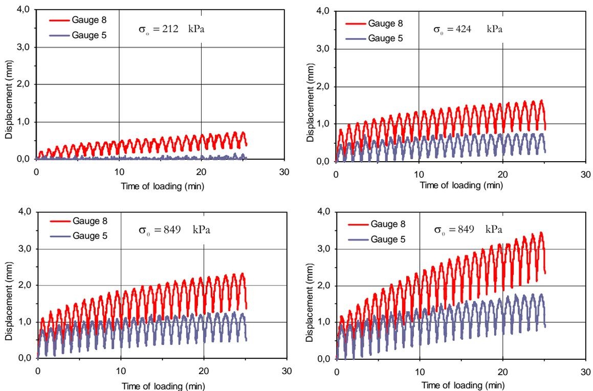
Figure 7: Displacements of gauge 5 (40 mm depth) and gauge 8 (80 mm depth) at 80mm base layer thickness and different vertical stresses amplitude  $\sigma_0$  with a frequency of 1Hz.
