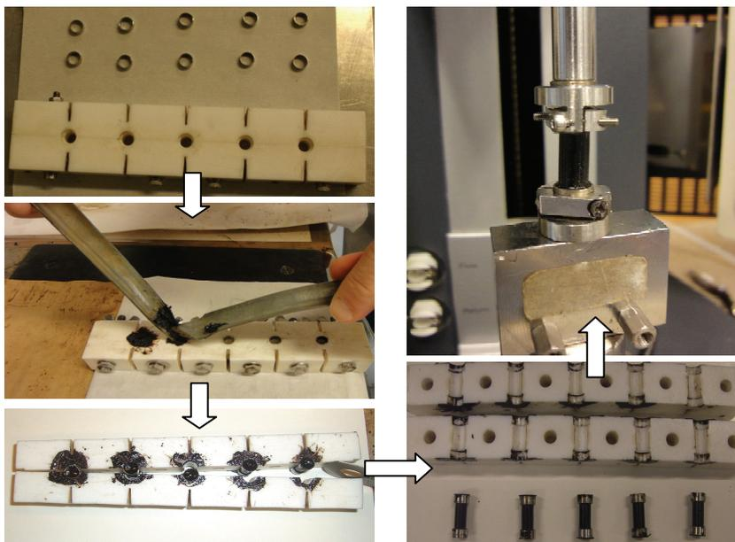
Figure 2: Illustration on sample preparation, extraction and test setup in the DSR
