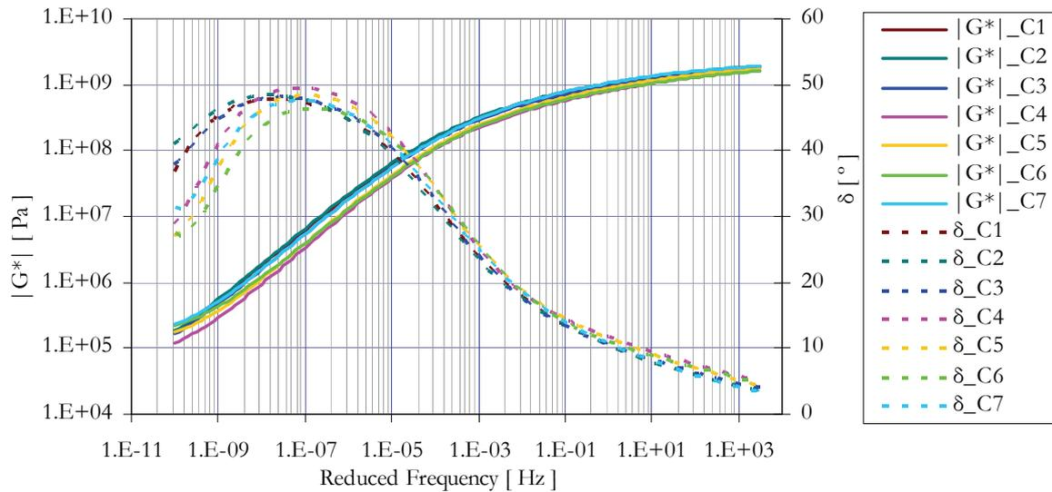
Figure 6: MC Comparisons at  $T_{ref} = -10^{\circ}\text{C}$ , mortars from binder C
