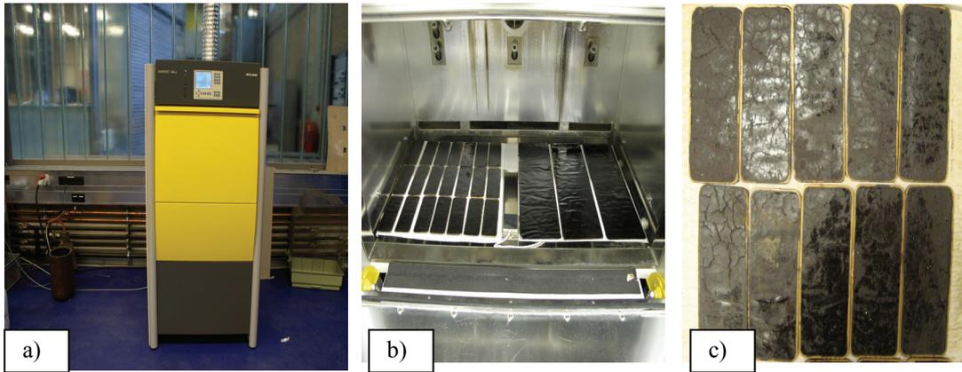
Figure1: Aging machine (a), 2mm thick mortar samples (b), aged mortar samples (c)
