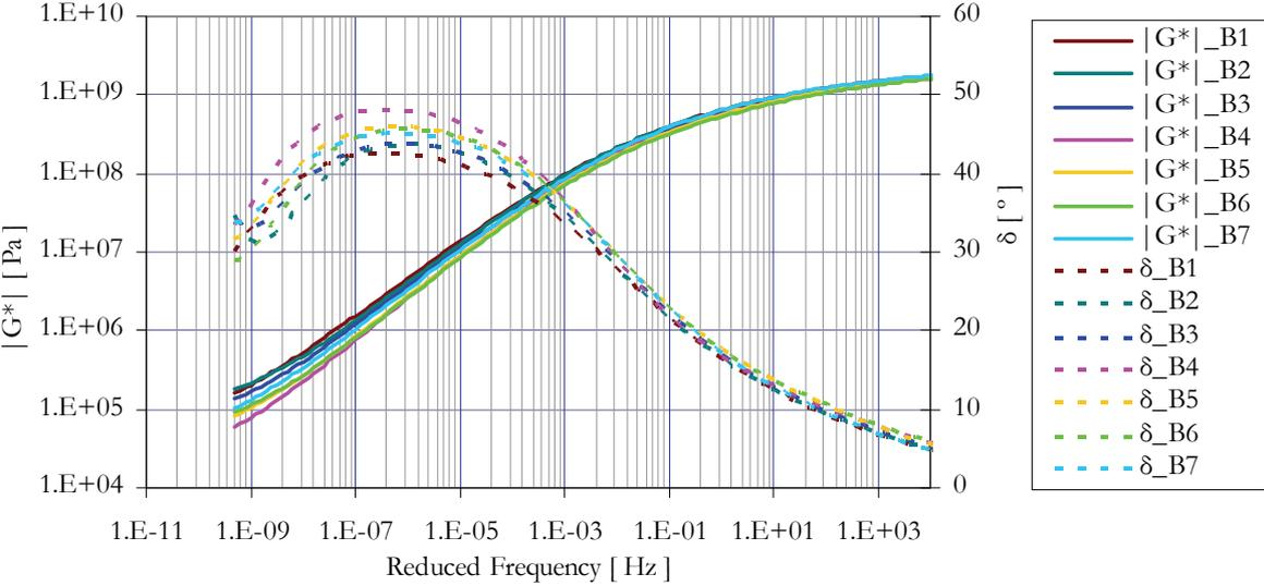
Figure 5: MC Comparisons at  $T_{ref} = -10^{\circ}\text{C}$ , mortars from binder B
