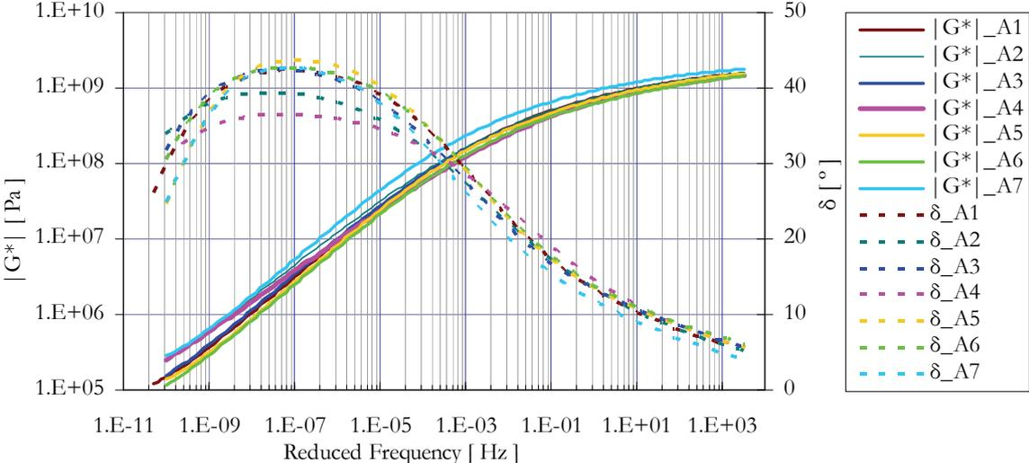
Figure 4: MC comparisons at  $T_{ref} = -10^{\circ}\text{C}$ , mortars from binder A
