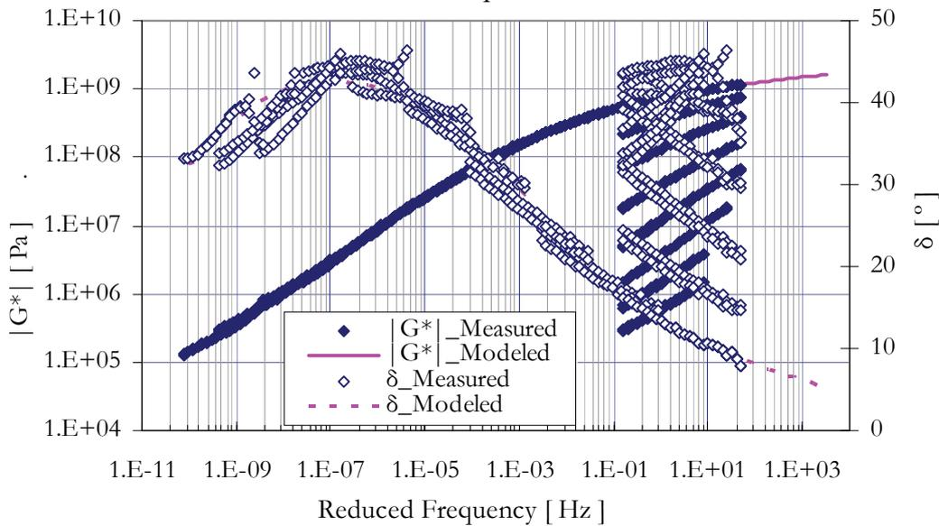
Figure 3: Master curve at a reference temperature of  $-10^{\circ}\text{C}$ , A1 mortar
