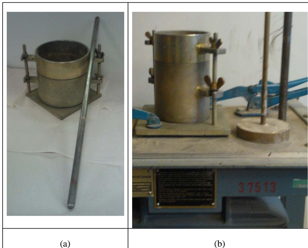
Figure 4: (a) Modified Proctor cylinder and steel rod, (b) Proctor cylinder, upper plate and vibrating table.
