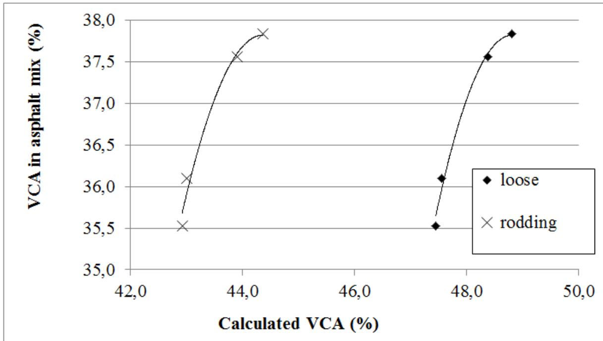
Figure 5: Skeleton density in the mix and calculated skeleton density
