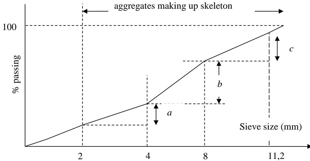
Figure 1: Aggregates making up the aggregate skeleton
