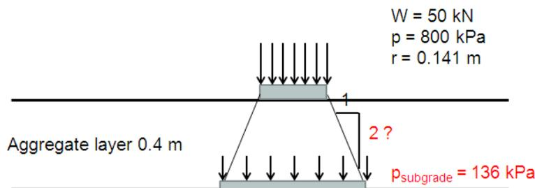
Figure 3: Assessment of vertical stress distribution based on the 1:2 distribution model.
