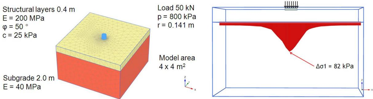
Figure 5: Distribution of vertical stresses predicted by the FE model shown on the left.
