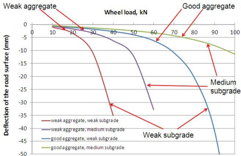
Figure 7: Examples of simulated load deflection curves obtained using the type of FE model shown in Figure 5.
