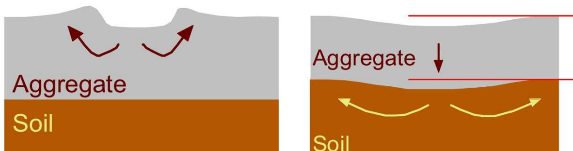
Figure 1: Mode 1 rutting (left) – shear deformation within the granular layers of the pavement near to the surface; Mode 2 rutting (right) – shear deformation within the subgrade with the granular layer following the subgrade (Dawson & Kolisoja 2004).
