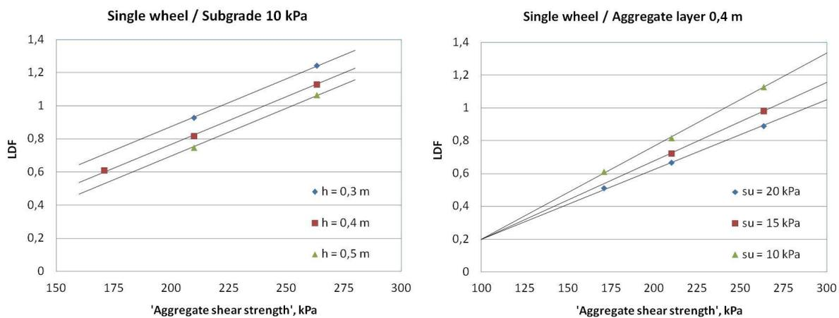
Figure 8: Load distribution factor, LDF, as a function of aggregate shear strength and aggregate layer thickness (left) and undrained shear strength of the subgrade soil (right).
