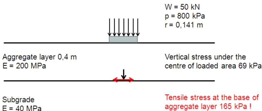
Figure 4: Example of multi-layer linear elastic modelling of a low volume road structure.
