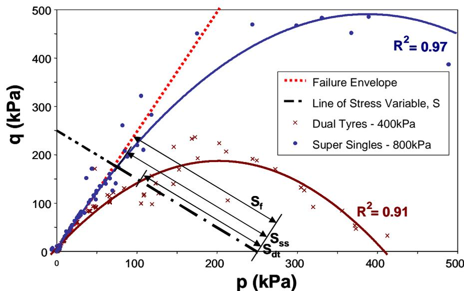
Figure2: Principle of the ‘proximity to failure approach’ (Dawson et al. 2007).
