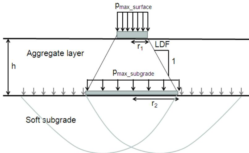
Figure 6: Basic idea of the suggested new design approach.
