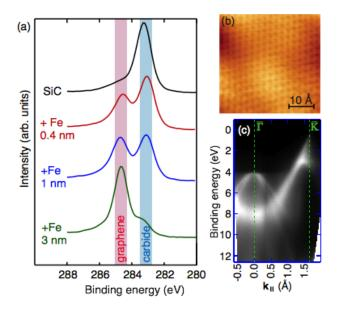
Figuretext: (a) XPS measurements of the carbide to graphene reaction, showing its dependence on the initial Fe quantity. (b) STM image of the graphene layer formed and (c) ARPES measurement showing the bandstructure of the graphene with its characteristic pi-band reaching a Dirac-point at K.
