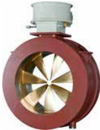
This picture shows a rim-driven thruster developed by Brunvoll
