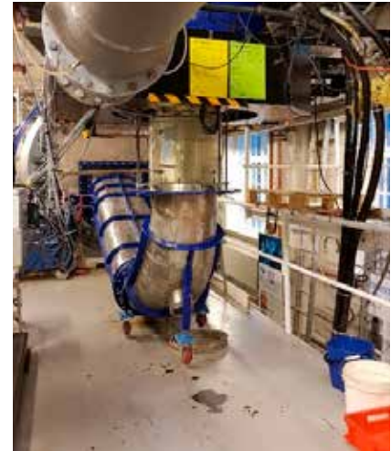
Francis rig at the Waterpower Laboratory at NTNU. Picture was taken during measurements.
