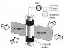
Stress measurement techniques. Hydraulic fracturing (Li, 2016)
