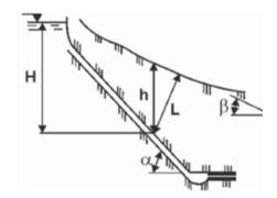
The illustration is related to the so-called Rules of thumb. The analytical stability assessment includes an assessment based on these design criteria (Panthi, 2014)
