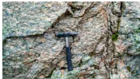
Figure 1 Corase grained granite in Roskrepp that will be tested in the laboratory.
