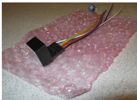
Figur 2.5 Strømregulator for LED
