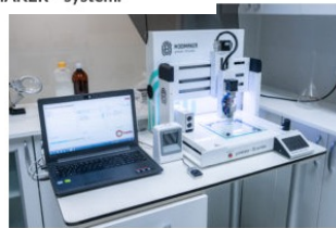
Figure 1: FabRx's M3DIMAKER™ 3D printing technology for personalised medicine production.
