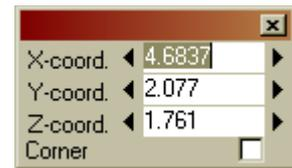
example the string @-0.2 is entered in the field for the y-coordinate, then all the y-coordinates of **all** selected points will be decreased by 0.20. So the y-coordinate for the displayed point becomes  $2.10 - 0.20 = 1.90$ . This is a convenient way to shift a number of selected points. If the project uses [imperial units](#) then it is also possible to enter a feet-inch/8 value as follows: 3-2-1, meaning 3ft 2 1/8 inch.
