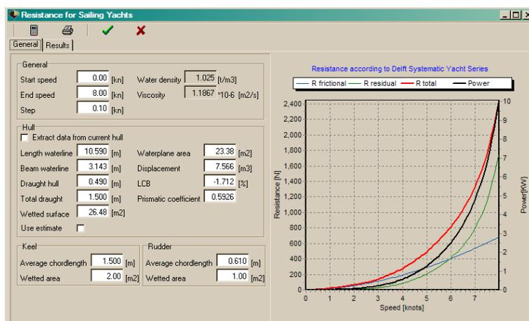
If there are no lines displayed in the graph to the right, then it's safe to assume that at least one of the parameters is out of range. You can switch to the results tab to check the details.
