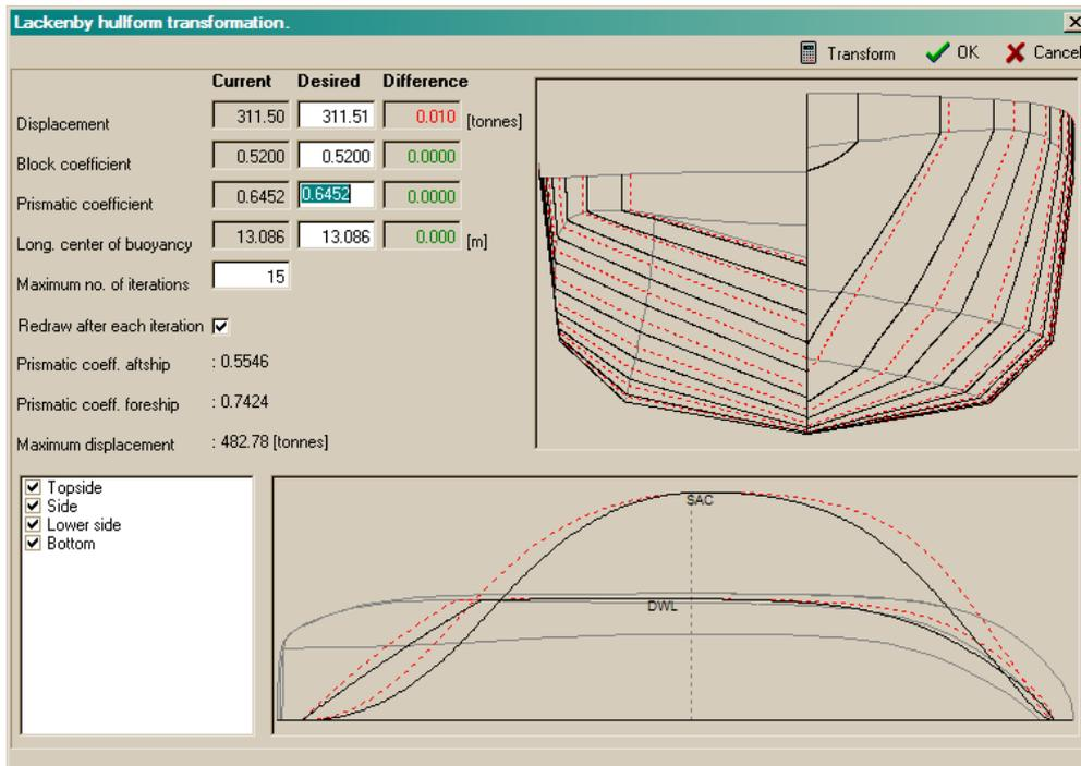
Here the result is shown after transforming the blockcoefficient from 0.4726 to 0.5200. The new lines and sectional area curve are displayed on top of the original lines.
