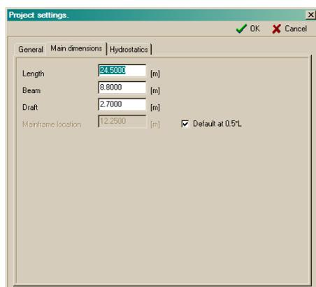
The second tab page is used to define the main particulars of the model, and the location of the midship section. By default this is at half the defined project length but this can be modified.
