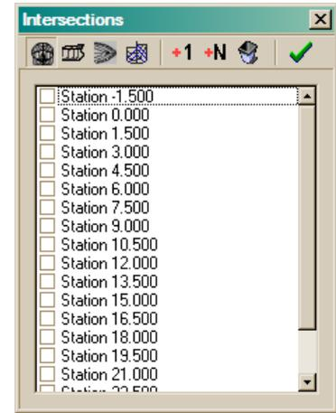
The checkbox displayed to the left of each intersection indicates if the curvature plot of that specific intersection curve must be plotted. (see [curvature visibility](#)). Due to the scale and nature of the computer screen it is in almost any case impossible to determine if a curve is fair. To overcome this
