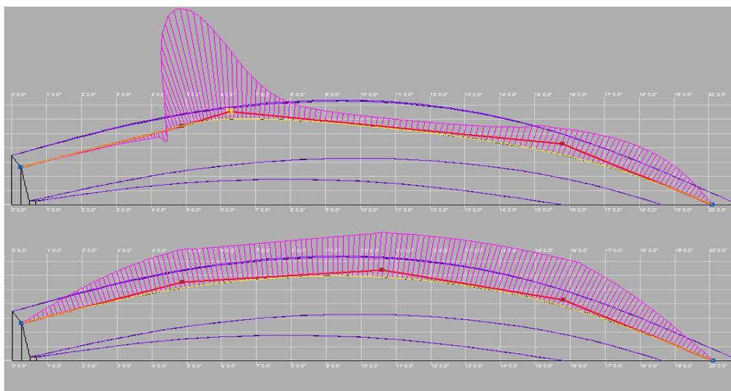
One thing to bear in mind is that the curvature at the first and the last point of the curve is always zero. This is due to the way the curve is being drawn, and it has nothing to do with the actual curvature of the surface at that point. Controlcurves are easier to fair when the controlpoints are spaced more or less evenly along the curve and are regular whenever possible. The less controlpoints a curve has, the easier it is to produce a good running smooth curve.
