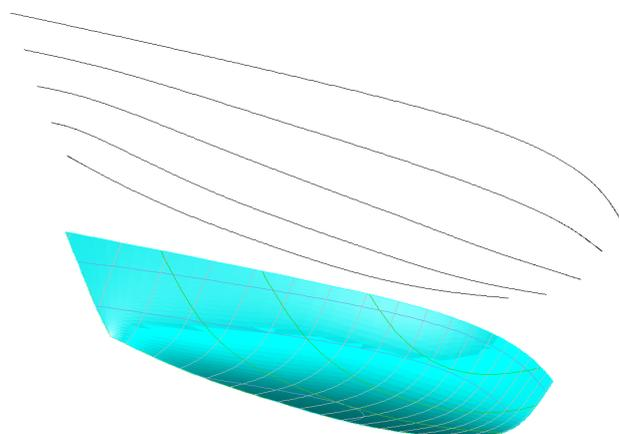
The user will be prompted how many points in longitudinal direction (number of columns) and in vertical direction (number of rows) the imported hull must have. Then the program fits a B-Spline surface through these points such that the new surface interpolates these points.
