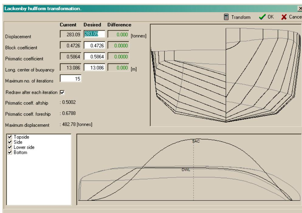
The input fields to the left are divided in 3 columns. The left column shows the current values as calculated from the model. The middle column shows the desired values which can be modified by the user. The right column shows the difference between the current and desired values. The left and right column are updated after each iteration so the progress can be monitored.
