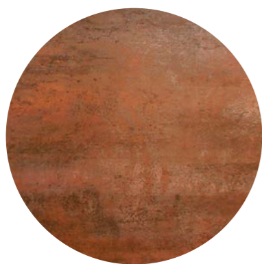
Corten steel cladding
