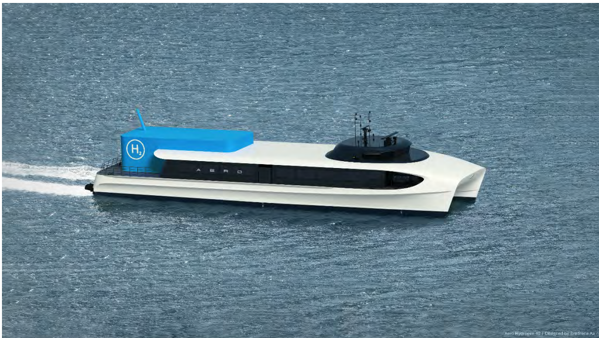
Aero 40 H2 fast ferry concept design by Brødrene Aa. Capacity for 277 passengers. Storage 4x154kg compressed hydrogen (figure: Brødrene Aa)
