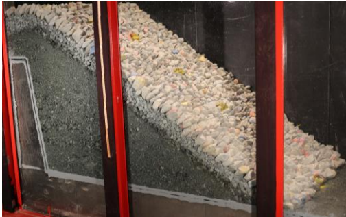
Rockfill dam with placed riprap
