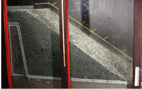
Rockfill dam without toe
