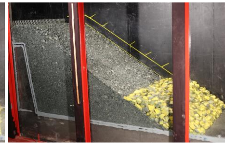
Rockfill dam with external toe
