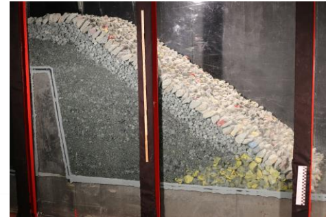
Rockfill dam with placed riprap and internal toe
