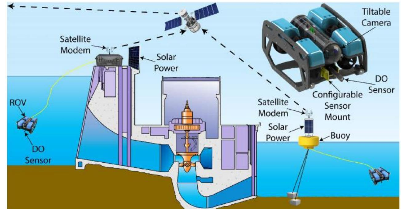
Figure 1. A visualization of the real-time and autonomous water quality monitoring system in operation.
