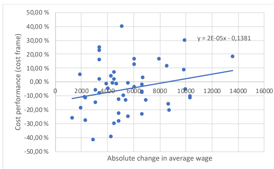
Figure 5.7 - Relation between cost deviation from the cost frame and the absolute change in average wage in the construction industry for road projects (N=50)
