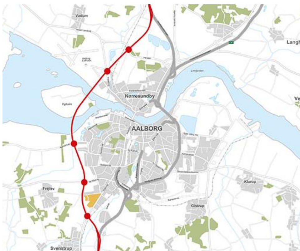
Figure 7.3 Limfjord Link, chosen alternative: Egholm Line, 20 km of new motorway west of Aalborg via the island of Egholm
