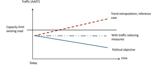
**Figure 8** Traffic development in different scenarios, illustrating that the need for an infrastructure project follows from the assumption that capacity should adapt to demand.
