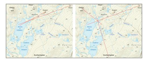
Figure 3-7: Poor triangulation (left) and good triangulation (right)
