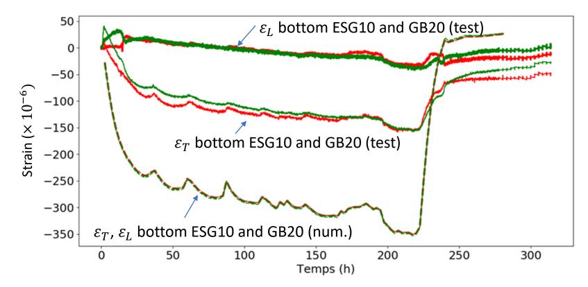
Computations for  $K_f = 0$  (temperature from 5 to -10 to 5°C)
