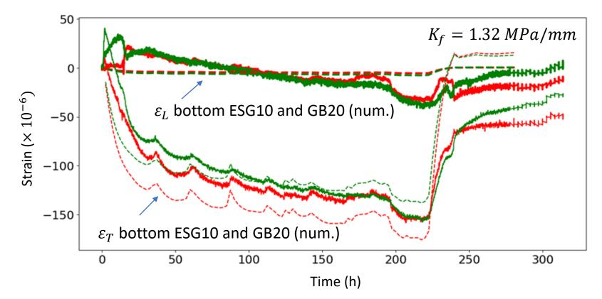
Computations for  $K_f = 1.32 MPa/mm$  (horizontal springs at bottom of GB20)
