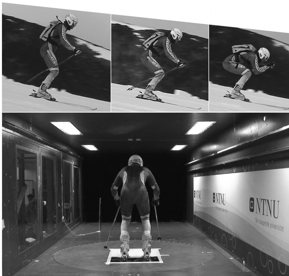
Fig. 1. The standard skiing positions (high, mid and low; top) and a skier standing in a midposition in the wind tunnel with a wind velocity of 60 km/h (bottom).
