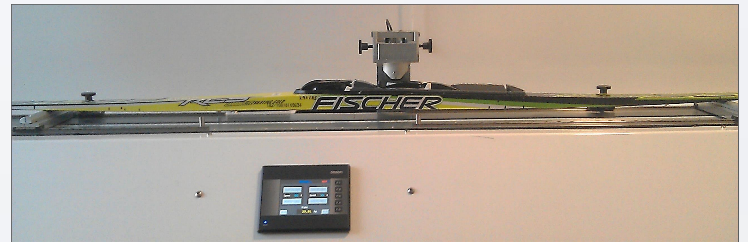
Figure 1: Developed ski test bench. Loaded ski during three point bending test.
