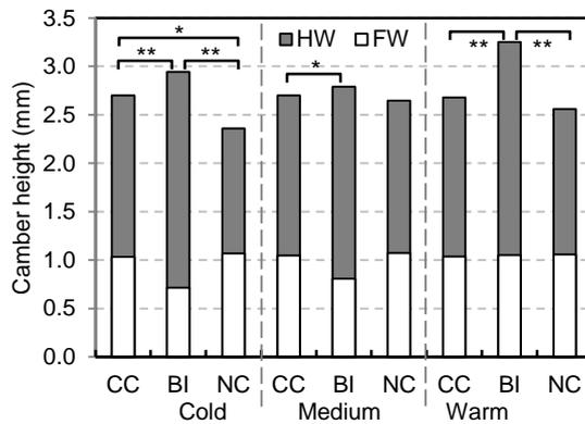
Figure C.2: Camber height at the balance point, loaded with *HBW* and *FBW* of the skiers. Significantly different between conditions at  $*P \leq 0.05$  and  $**P \leq 0.01$ .
