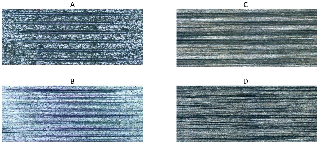
Figure G.5: Sample surface textures from metal cutting (A, B) and stone grinding (C, D), the image size is  $2.16 \text{ mm} \times 5.25 \text{ mm}$ .
