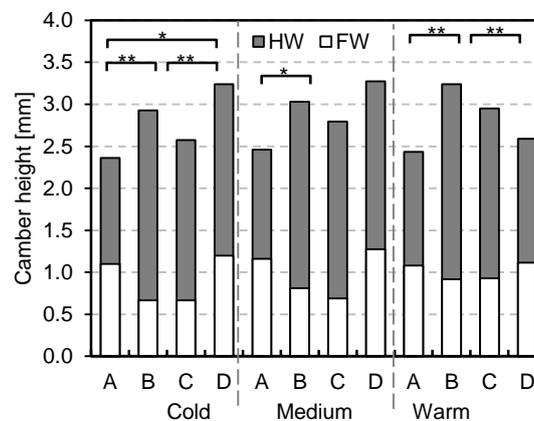
Figure 4.6: Camber height measured at balance point loaded with half and full BW for all four ski brands and temperature categories, with significant difference between conditions at  $*p \leq 0.05$  and  $**p \leq 0.01$ .
