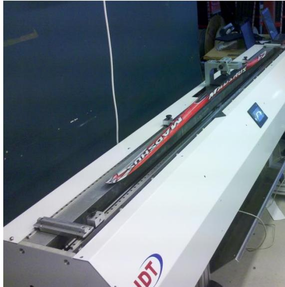
Figure 3.2: Ski Analyzer, the developed ski test bench in cooperation with IDT AS, Lena.
