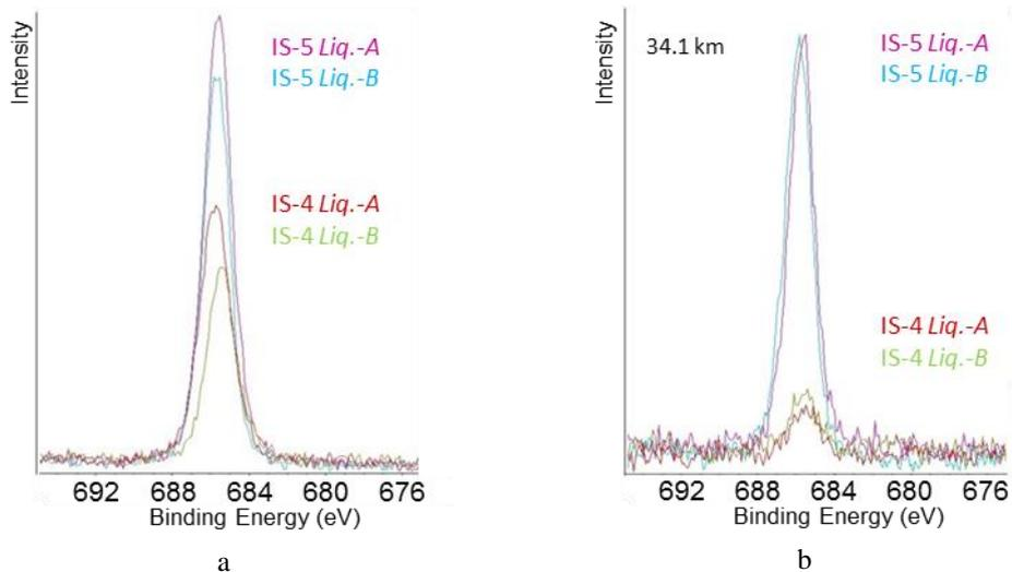
Figure F.1: (a). XPS analyses from both base materials compared with Liq.-A and Liq.-B wax before skiing and (b) after skiing 34.1 km (in the spectra F 1s).
