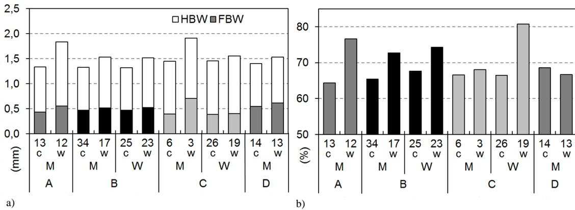
Figure D.2: a) Camber Height at the balance point for all four ski brands (A – D), both gender groups (M, W) and temperature categories (*cold* and *warm*). b) Average load which is necessary to compress the ski down to 0.2 mm camber height as fraction of the skier's body weight.
