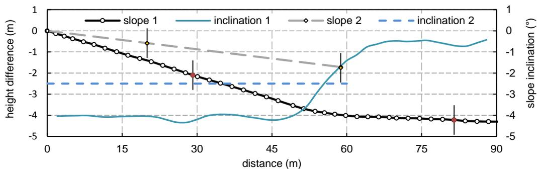
Figure E.3. Slope and inclination from test Tracks 1 and 2. The location of both photo cell units is marked with vertical black bars.
