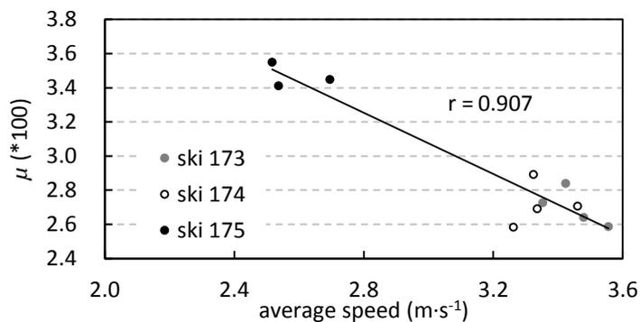
Figure E.8: Average speed versus calculated coefficient of friction,  $\mu$  for each heat and ski with a linear regression line in black to the right.
