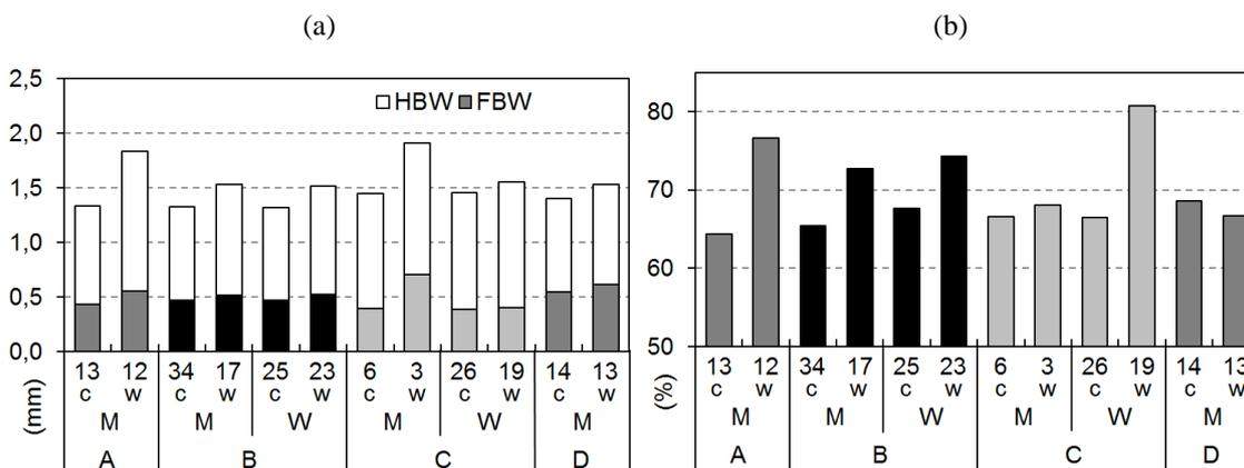
Figure 4.4: a) Camber height at the balance point for all four ski brands (A – D), both gender groups (M, W) and temperature categories (*cold* and *warm*); b) Average load necessary to compress the ski down to 0.2 mm camber height as a fraction of the skier's body weight.
