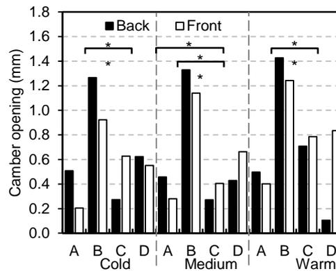
Figure C.4: Camber opening height measured with *FBW* at  $\pm 41.6\%$  of the ski length in front (white) of and behind (black) the *BP*. Significantly different between conditions at  $*P \leq 0.05$  and  $**P \leq 0.01$ .
