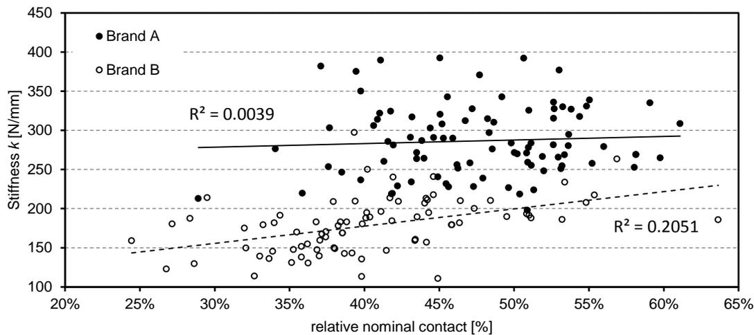
Figure 4.7: Ski camber stiffness as a function of the relative nominal contact length for two selected ski brands. All measured skis are plotted. Linear regression lines are drawn in the figure.
