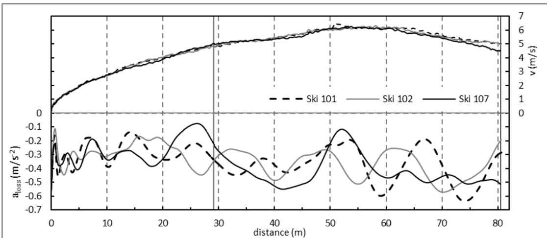
Figure 4.16: Results from the inertial measurement unit (Test 1, Heat 3). The two photocell units are marked with vertical black lines at 29.5 m and 80.2 m into the test track.
