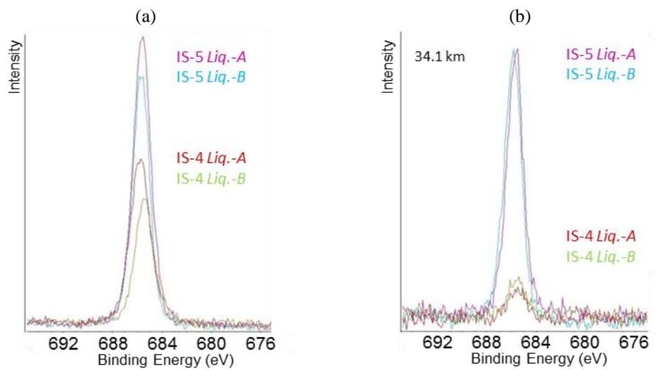
Figure 4.19: (a). XPS analyses from both base materials compared with Glider-A + Liq.-A and Liq.-B wax before skiing and (b) after skiing 34.1 km (in the spectra F 1s).
