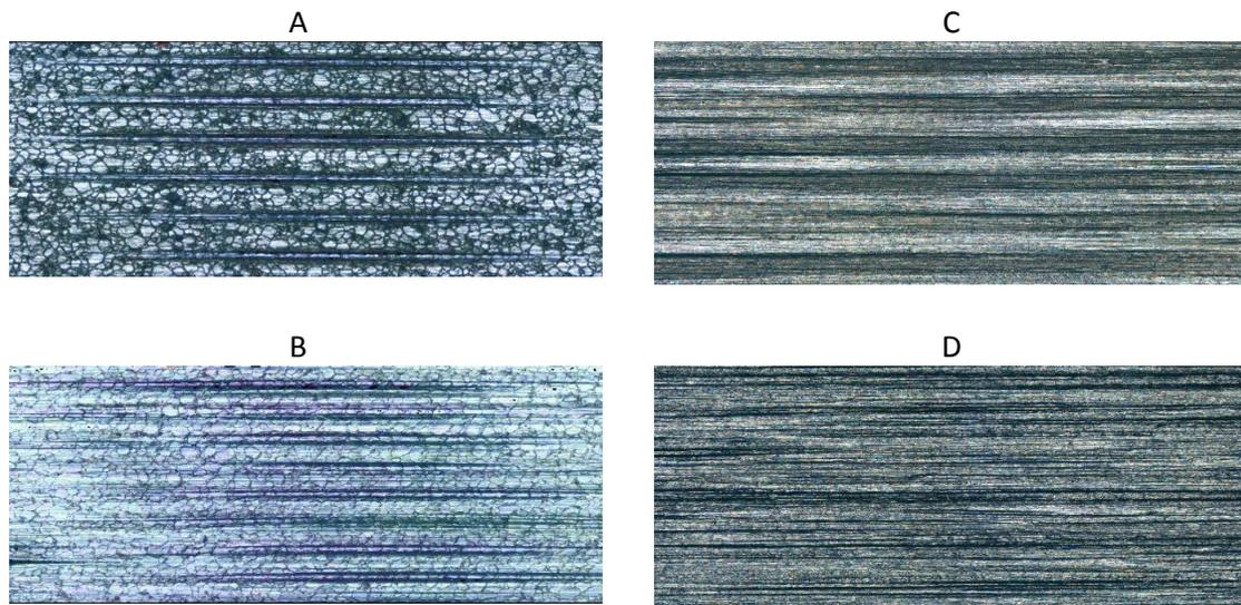
Figure 4.9: Sample surface textures from metal cutting (A, B) and stone grinding (C, D), the image size is 2.16 mm  $\times$  5.25 mm.
