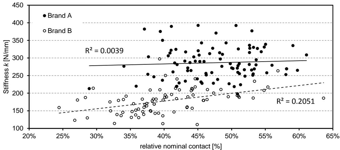
Figure C.7: Ski camber stiffness as a function of the relative nominal contact length for two selected ski brands. All measured skis are plotted. Linear regression lines are drawn in the figure.
