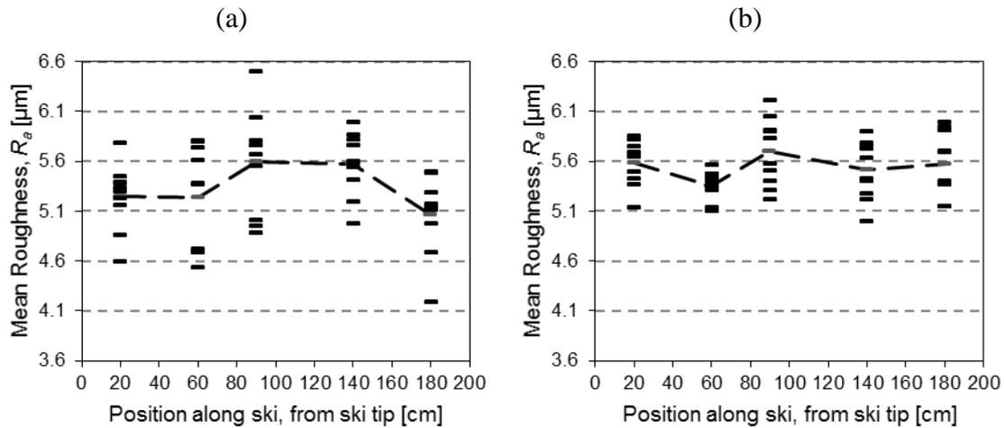
Figure G.7: Mean roughness,  $R_a$  results for all measurement points along the five chosen points along the ski. The average of each point is connected with a dashed line; (a) stone ground skis and (b) metal ground skis.
