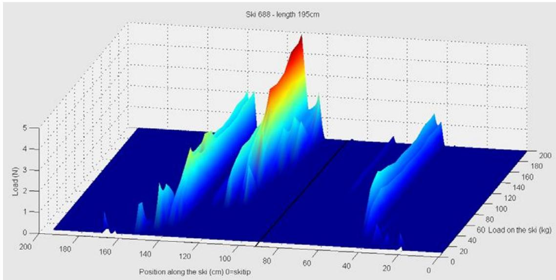
Figure 2.4: Load distribution along a ski for applied static loads ranging from 0 kg to 200 kg (Breitschädel, 2007).
