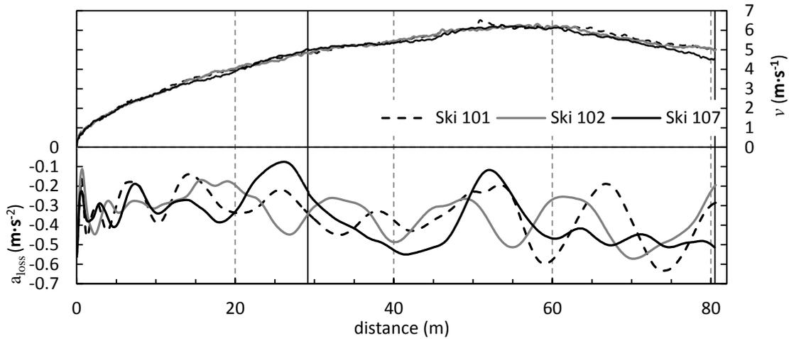
Figure E.6: Results from the inertial measurement unit (Test 1, heat 3). The two photocell units are marked with vertical black lines at 29.51 and 80.15 m into the test track.
