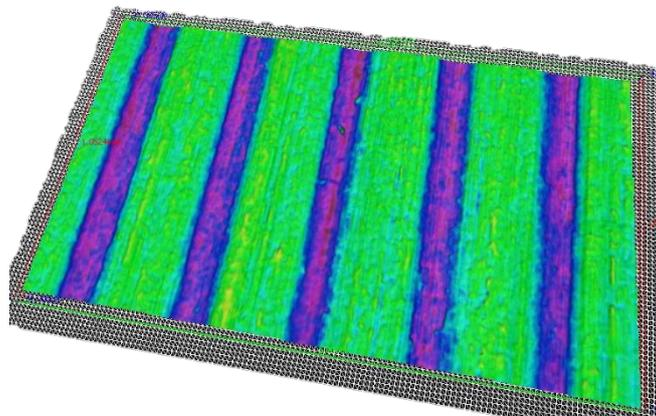
Figure G.2: An example of a linear stone ground structure on a ski, picture taken with an Alicona 3D microscope.
