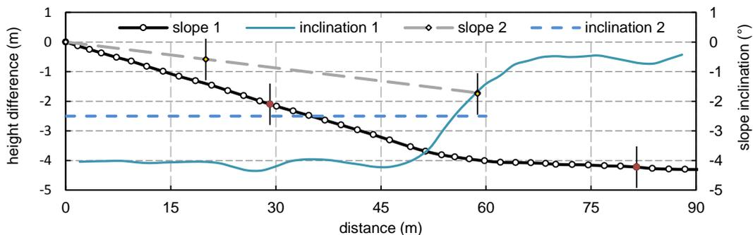
Figure 3.7: Slope and inclination from test Tracks 1 and 2. The location of both photo cell units is marked with vertical black bars.
