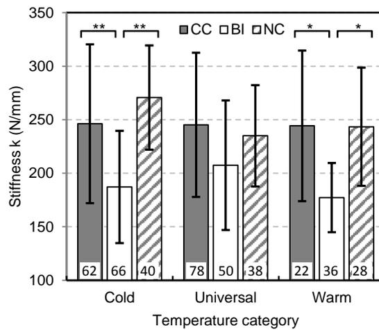
Figure C.1: Mean camber stiffness for all measured skis from CC, BI and NC split into three temperature categories. Significantly different between conditions at  $*P \leq 0.05$  and  $**P \leq 0.01$ .
