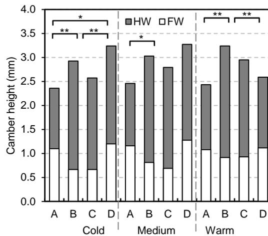
Figure C.6: Camber height measured at balance point loaded with half and full weight for all four ski brands and temperature categories. Significantly different between conditions at  $*P \leq 0.05$  and  $**P \leq 0.01$ .
