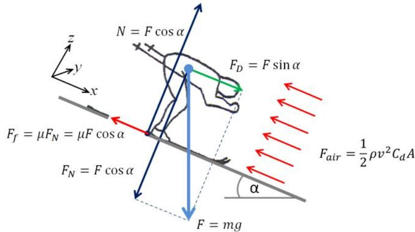
Figure E.1: Simplified forces which act on a skier in a straight downhill, modified sketch from (Spring, 1989).
