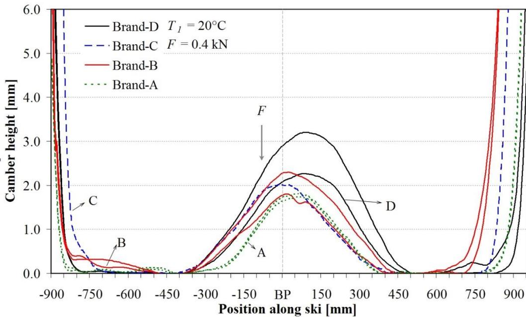
Figure A.1: The different Span-curves for all measured skis at the  $T_1$  loaded with  $F = 0.4$  kN. On the horizontal axis is the position along the ski with the rear ski end at about  $-900$  mm and with the balance point (BP) at  $0$  mm. Camber height is on the vertical axis in mm.
