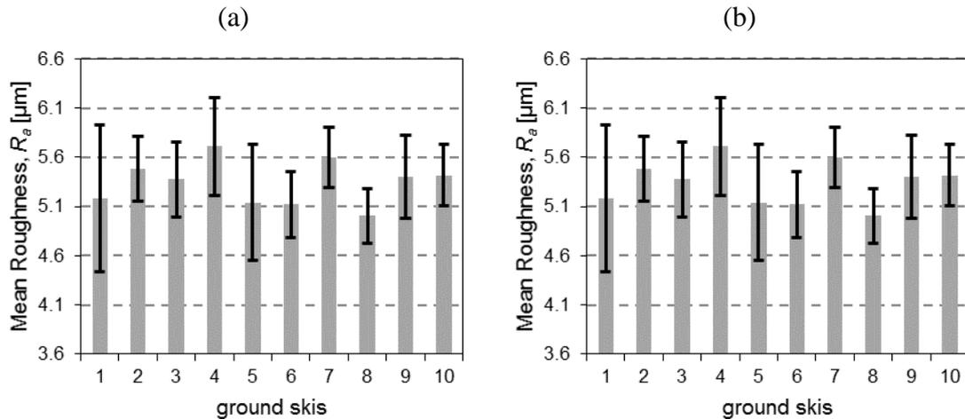
Figure G.9: Average mean roughness,  $R_a \pm \sigma$  for the ten ground skis; (a) stone ground skis and (b) metal ground skis.
