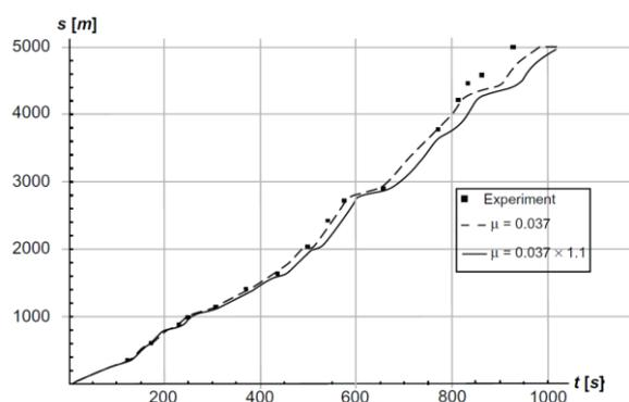
Figure 2.5: Simulated and experimental positions  $s$  in meters as a function of time  $t$  in seconds along a track while skiing on snow using the skating technique. Dashed line:  $\mu = 0.037$ ; Solid line:  $\mu = 0.037 \times 1.1$  (Moxnes et al., 2013).
