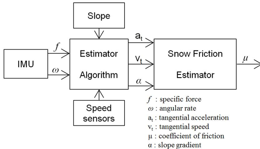
Figure E.2: Schematic sketch of the model design for the IMU system (E).
