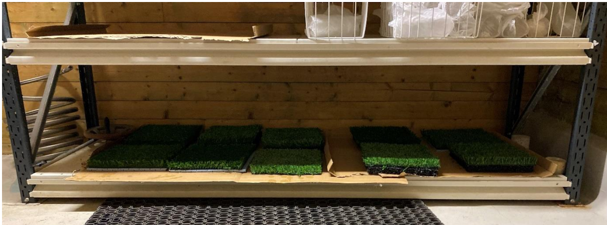
Figure 7: The figure show where the ten samples were placed inside of the conditioning cabinet. A cardboard is placed underneath the samples to avoid freezing into the metal shelves.
