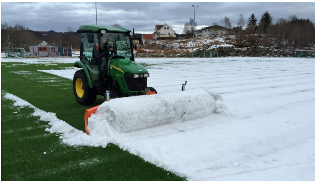
Figure 3: Rolling the snow during snow removal prevents damage to the fibers [13].
