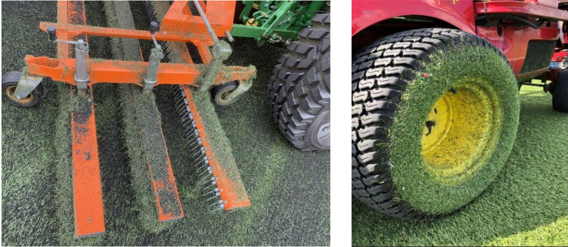
Figure 1: Loose fibers piled up on maintenance equipment. Photo by Bjørn Aas.
