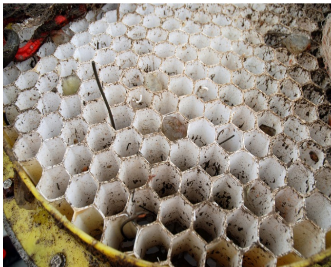
Figure 42 – Sediment trap's honeycomb baffle in 2012 after one year on the seabed. Photo: NTNU Vitenskapsmuseet
