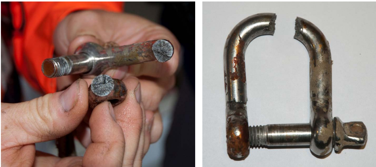
Figure 28 – Broken shackle from sediment trap rig, 2008. Photo: NTNU Vitenskapsmuseet
