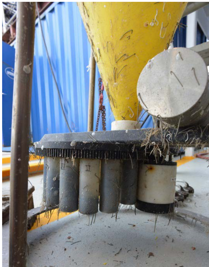
Figure 15 – The lower part of the sediment trap with the sample bottles, controller housing and stepper motoring housing. Photo: NTNU Vitenskapsmuseet
