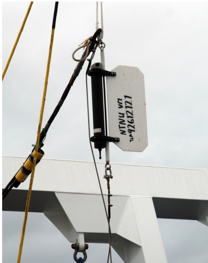
Figure 18 - Nortek Aquadopp fitted with Aquafin. On the left is a transponder fitted to the wire to monitor the position of the rigging during deployment and re-deployment of the instrument rig. Photo: NTNU Vitenskapsmuseet
