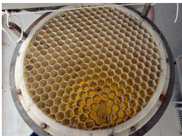
Figure 14 – Topside view of the funnel's honeycomb baffle. Photo: NTNU Vitenskapsmuseet
