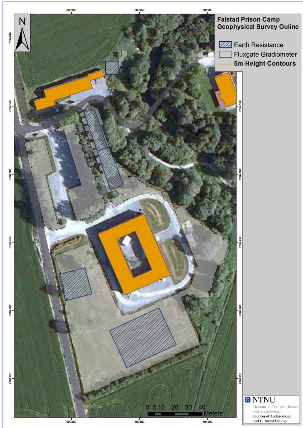
Figure 13: The figure shows the areas surveyed with an earth resistance meter and by fluxgate gradiometer.
