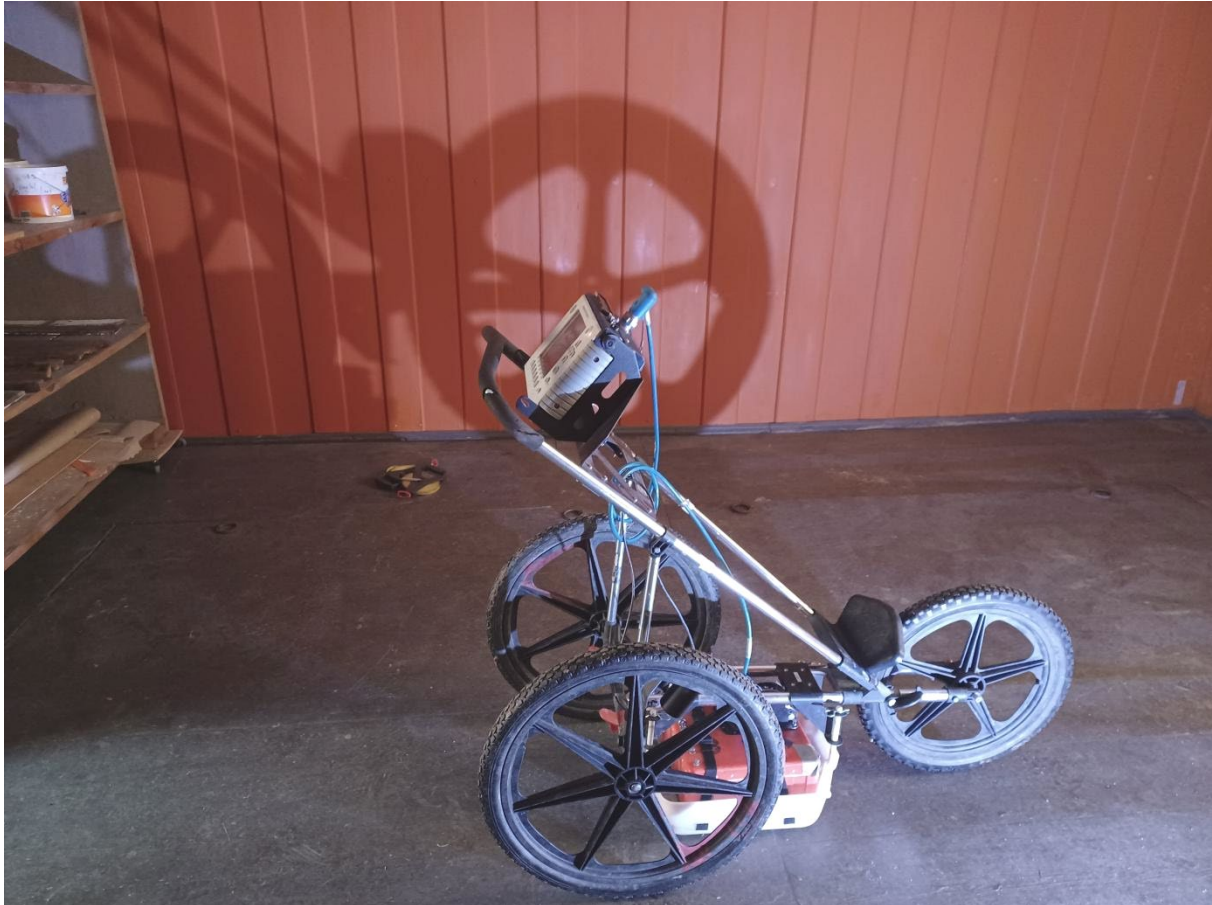
Figure 2: Foto taken within the chapel during the GPR investigation.
